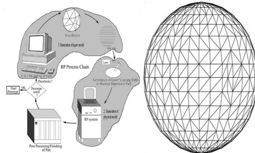
**Figure 1:** RP process chain and tessellation of a sphere [3]
