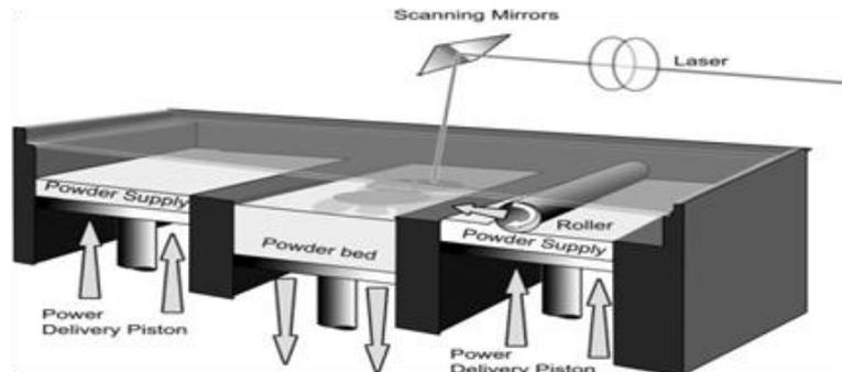
Figure 6: working of selective laser sintering [6]
