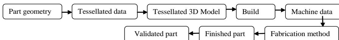
**Figure 3:** Design process of RP
