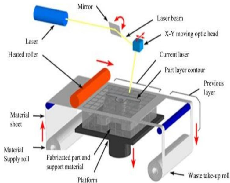
**Figure 8:** working of laminated object manufacturing [8]
