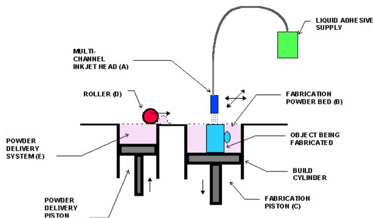
Figure 7: working of three dimensional printing [7]
