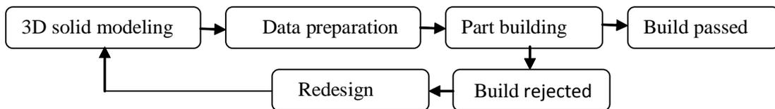
**Figure 2:** Process cycle
