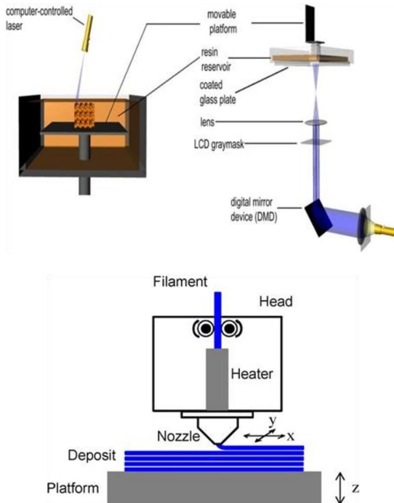
**Figure 4:** Block diagram of Stereolithography [4] **Figure 5:** Block diagram of fused deposition modeling [5]
