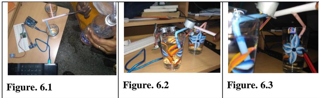
**Figure 6.1** shows that the water is flowing from the Main tank and supplied to the first water tank through pipe. After the certain level has reached the water is sensed through the ultra sonic sensor and supply of water is stopped using stepper motor (**figure 6.2**). Now, the flow of water turned to next water tank (**figure 6.3**).
