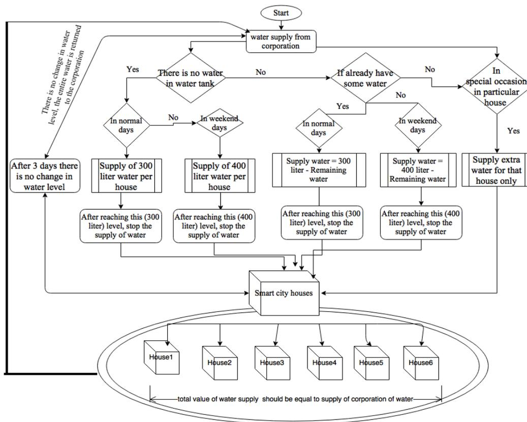
Figure. 2. Flow diagram for proposed system
