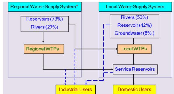
**Figure. 1.** Structure of water supply management system
