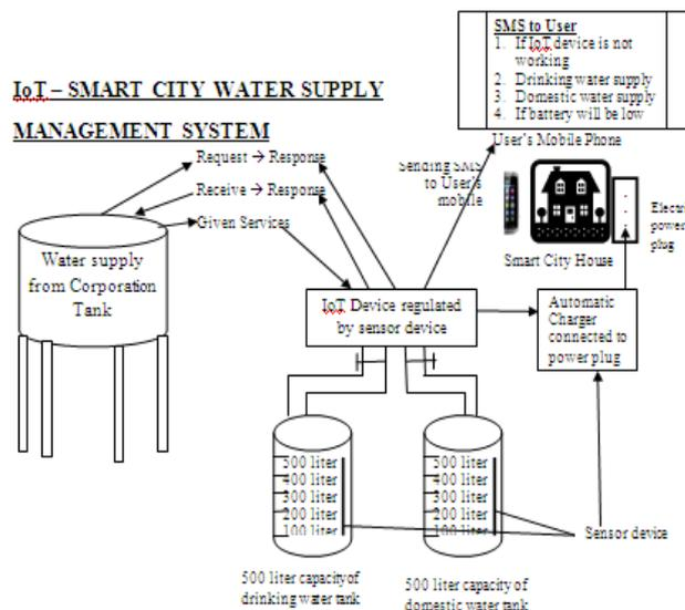
**Figure. 3.** Block diagram for proposed system
