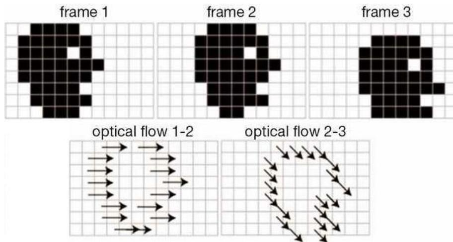
**Fig 2:** Optical flow of frames [5]
