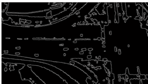
Figure 4: Canny edge detection
