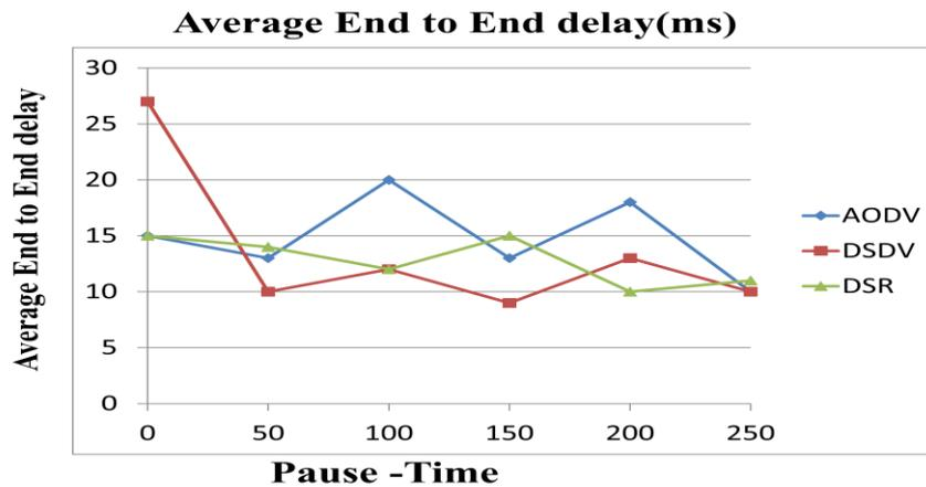
**Figure 2.** Avg. end to end delay versus pause time for AODV, DSR and DSDV (Number of node = 50, Area space = 500m x 500m)
