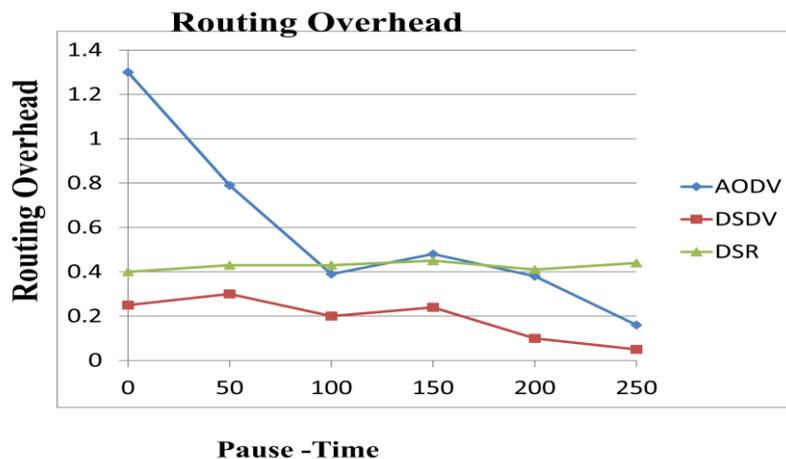
**Figure3.** Routing overhead versus pause time for AODV, DSR and DSDV (Number of node = 50, Area space = 500m x 500m)
