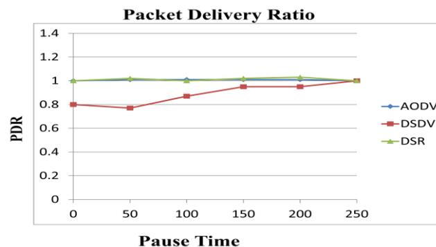
**Figure 1.** Packet delivery ratio versus pause time for AODV, DSR and DSDV (Number of node = 50, Area space = 500m x 500m)
