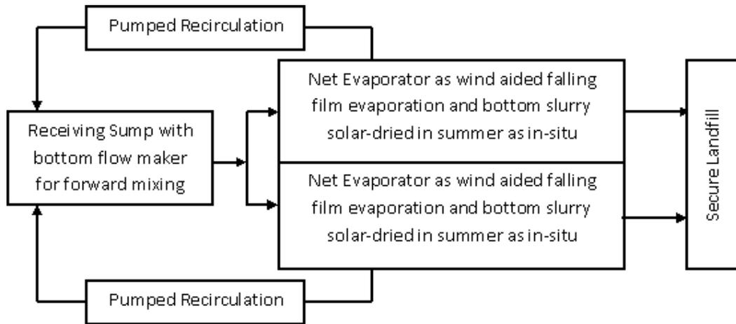
**Figure 3:** Schematic of the Demonstrated Alternative System for High TDS Wastewaters
