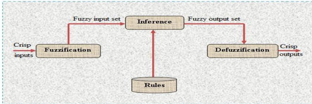
**Fig.2** Architecture of Fuzzy Logic System
