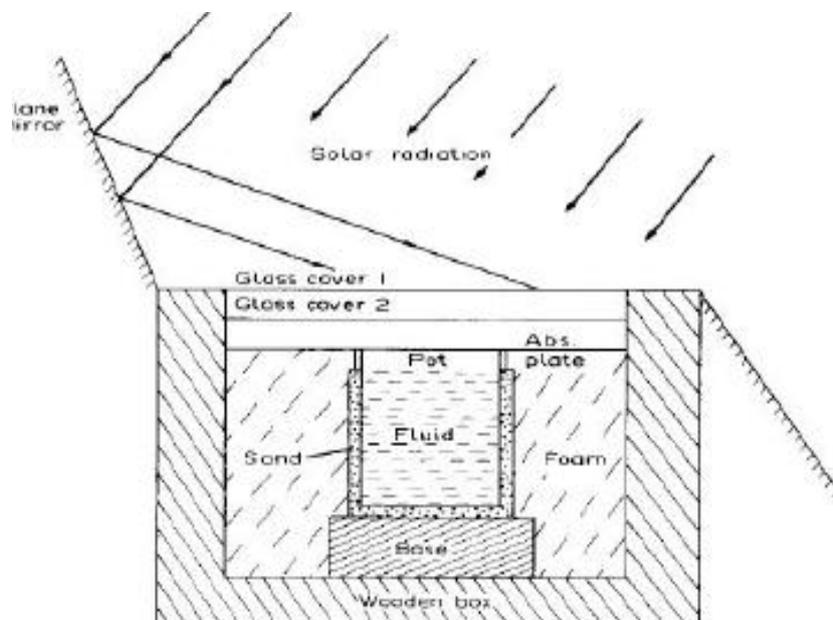
**Figure 6:** Solar cooker with sand
