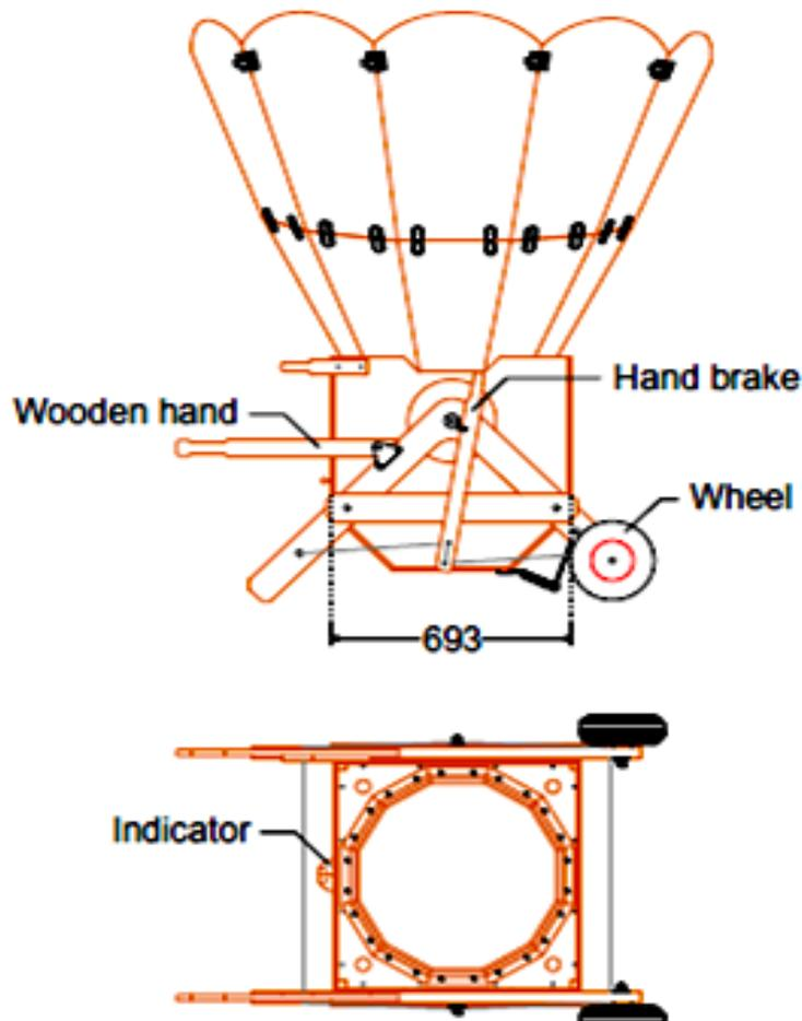
Figure 1: Solar box type cooker
