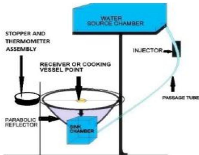
**Figure 7:** Parabolic dish type solar cooking system with gravity based solar tracking system
