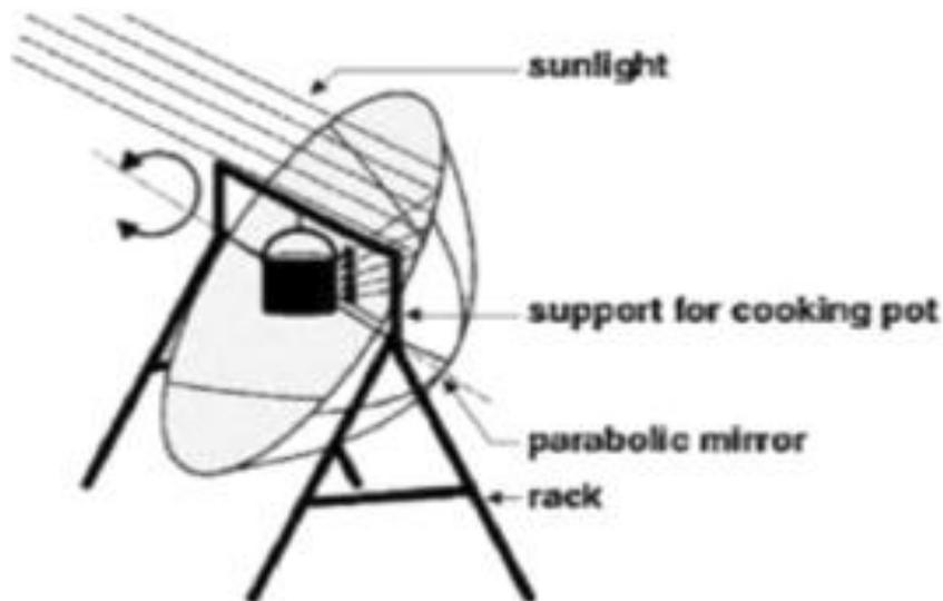
**Figure 4:** Concentrating type solar cooker
