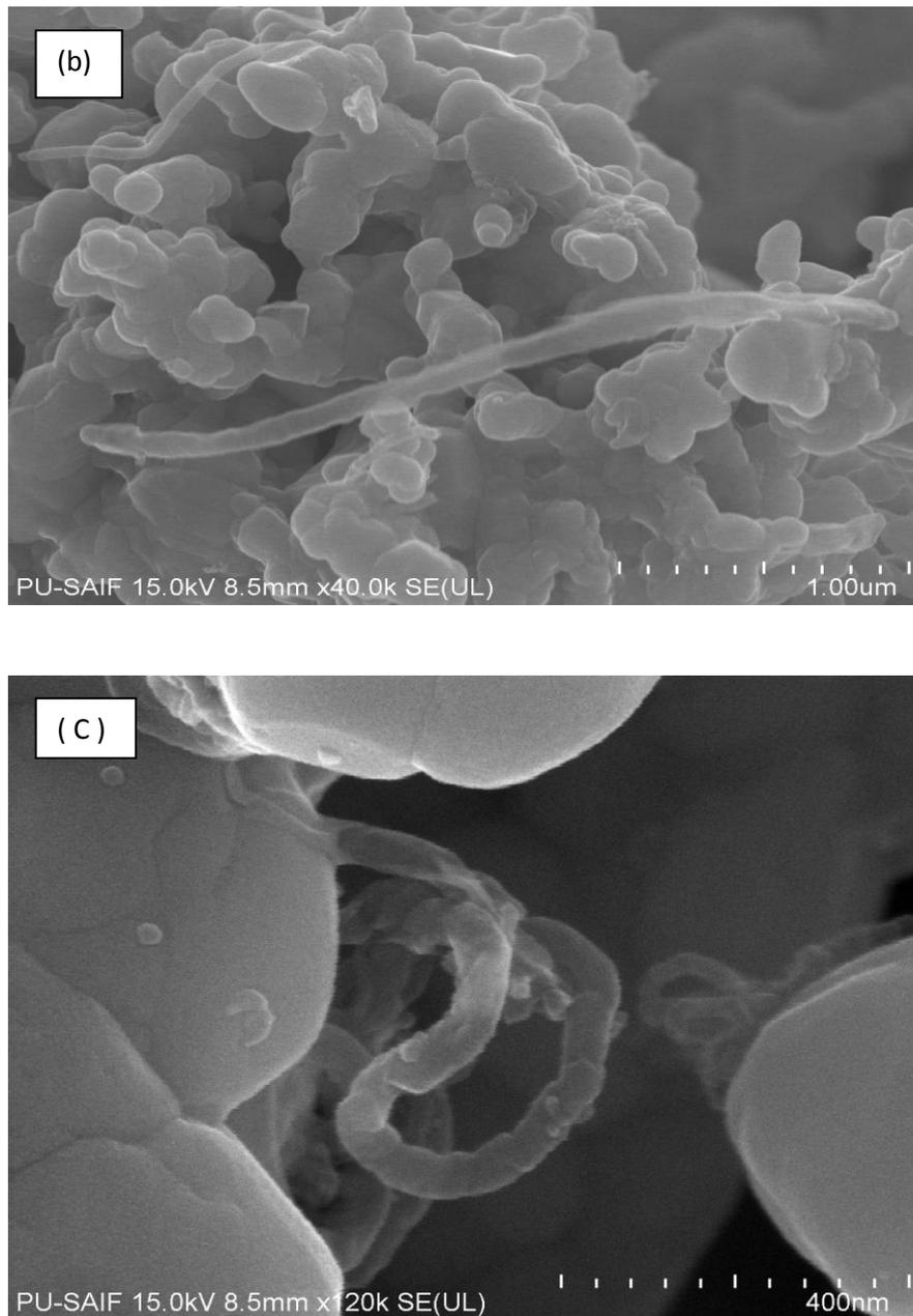
**Figure 3.** SEM micrographs of (a) CNT (1.5 vol. %) /Ag, (b) CNT (3 vol. %) /Ag and (c) CNT (4.5 vol. %) /Ag
