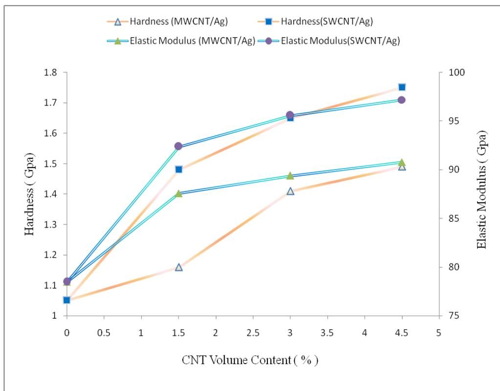
**Figure 5.** Variation of Hardness and Elastic Modulus of CNT/Ag nanocomposite with variation in CNT volume Content after sintering.
