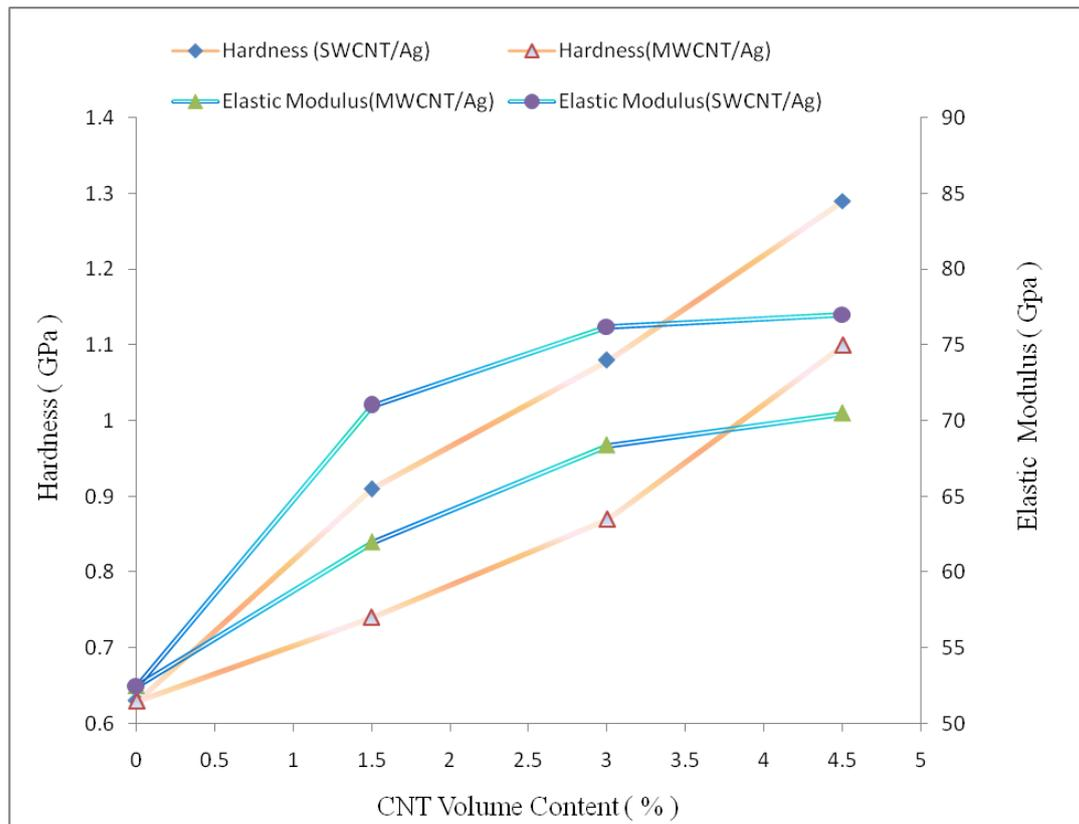
**Figure 4.** Variation of Hardness and Elastic Modulus of CNT/Ag nanocomposite with variation in CNT volume Content before sintering.
