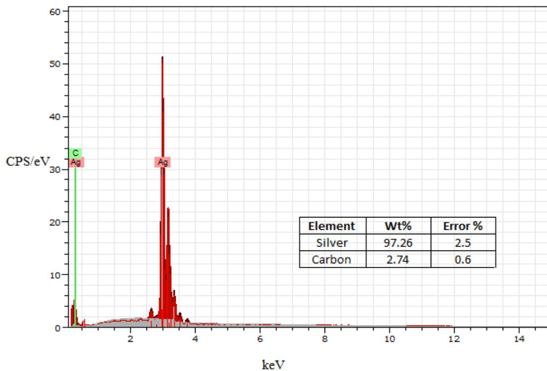
**Figure 2.** EDS characteristic profile of CNT/Ag Nanocomposite
