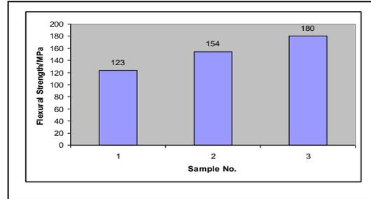
**Fig. 3.4** Flexural strength of cotton-ramie fabric reinforced composites
