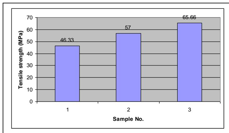
**Fig. 3.1** Tensile strength of cotton-ramie fabric reinforced composite
