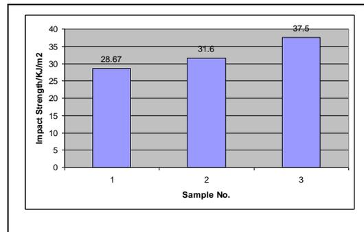
**Fig. 3.6** Impact strength of cotton-ramie fabric reinforced composite
