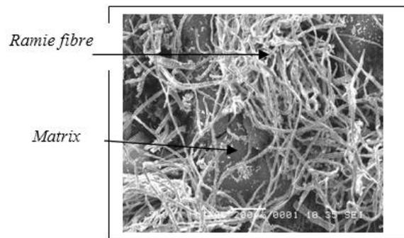
**Fig. 3.3** Surface Image after breakage on Tensile Test
