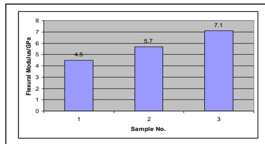
**Fig. 3.5** Flexural modulus of cotton-ramie fabric reinforced composite
