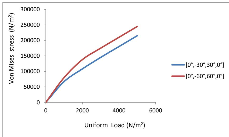
Fig:2- Von Mises stress vs Uniform Load
