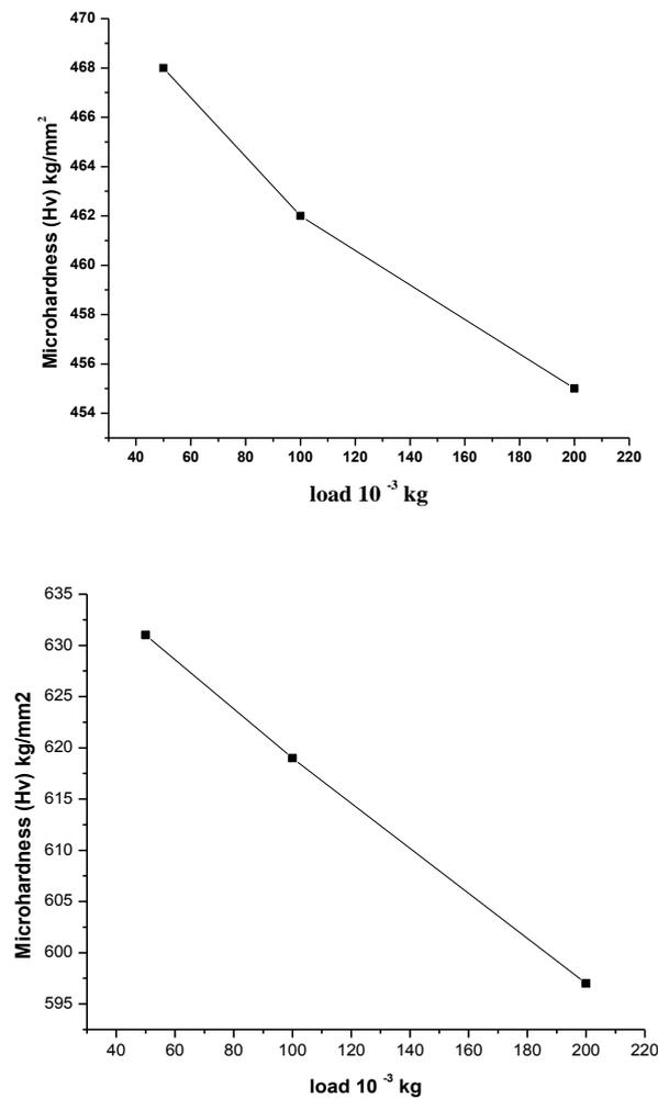
**Figure 4.** Microhardness vs. Load for BTB-6 and BSB-6 Glass
