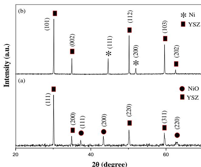
**Fig. 1** XRD pattern of (a) YSZ/NiO composite and (b) YSZ/Ni cermet.
