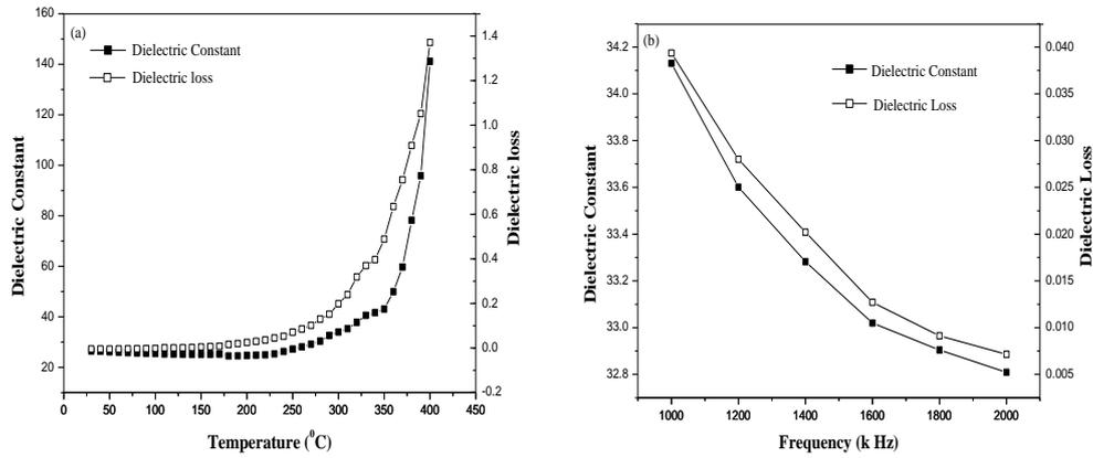
**Fig. 5** (a) Temperature versus Dielectric constant and Dielectric loss at frequency 1 MHz for YSZ/NiO sintered sample (b) Frequency versus Dielectric constant and Dielectric loss at temperature 500 K for YSZ/NiO sintered sample.
