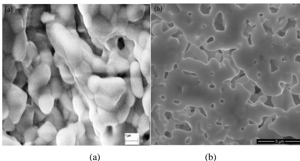
**Fig. 2** SEM micrograph of (a) YSZ/NiO composite sintered at 1350 °C for 5 hr and (b) reduced YSZ/Ni cermet.
