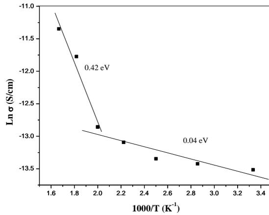
**Fig. 6** Arrhenius plot for conductivity of sintered YSZ/NiO composite at frequency 2 MHz.
