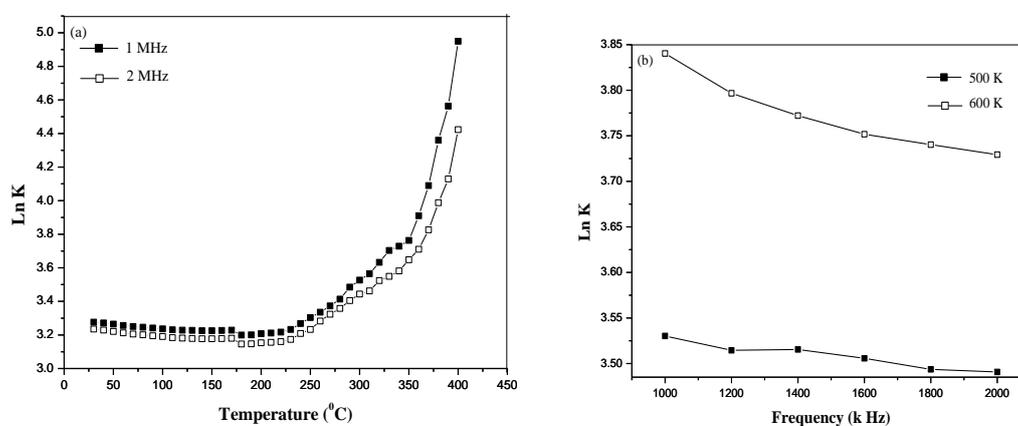
**Fig. 4** (a) Temperature and (b) Frequency dependent behavior of dielectric constant in YSZ/NiO sintered composite.
