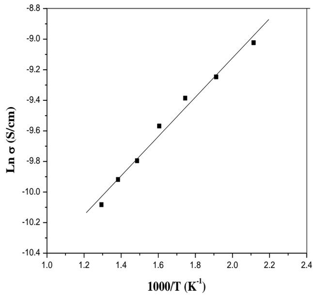
**Fig. 8** Electrical conductivity of YSZ/Ni anode cermet as a function of temperature.
