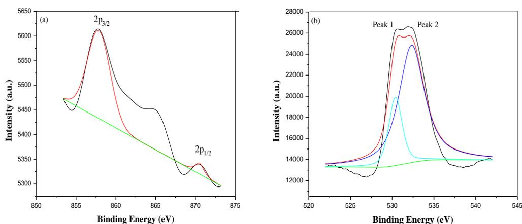
**Fig. 3** XPS spectrum of (a) Ni(2p) and (b) O(1s) in YSZ/NiO sintered sample.
