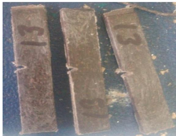
Figure: 4. Impact testing samples after V- Notching.
