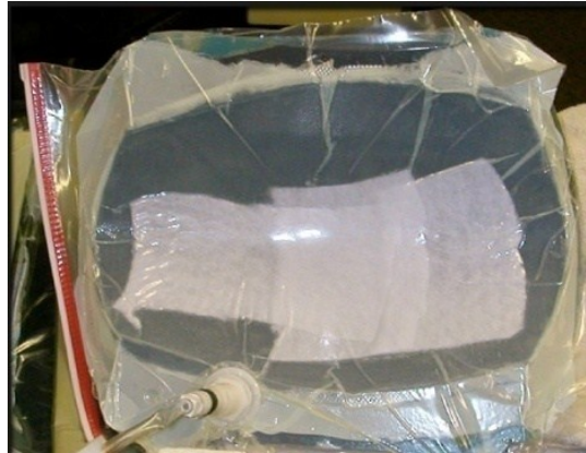
Figure 12. Vacuum Bag technique
