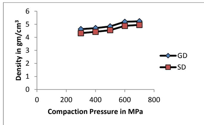
**Figure 2:** Green density and 850<sup>o</sup>C sintered density of the processed material at various compaction pressures.
