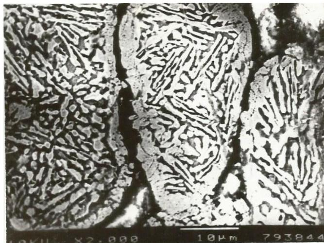
**Figure 5:** SEM micrograph of surface decarburized high carbon content rapidly solidified alloyed ferrous powders
