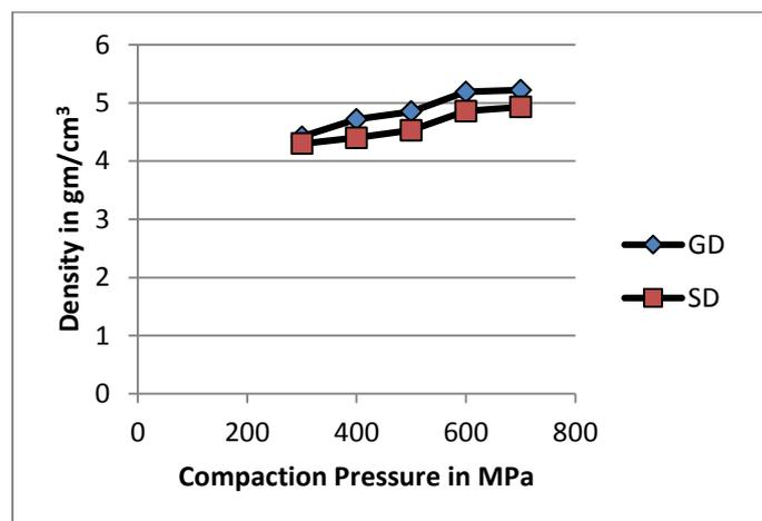
**Figure 3:** Green density and 1000<sup>o</sup>C sintered density of the processed material at various compaction pressure
