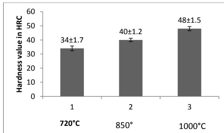
**Figure6:** Hardness values of processed materials compacted all at 700MPa and sintered at 720<sup>0</sup>C,850<sup>0</sup>C &1000<sup>0</sup>C.
