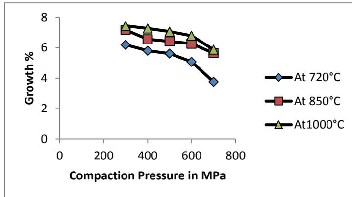
**Figure 4:** Growth % of the processed material at various sintering temperatures and compaction pressures.
