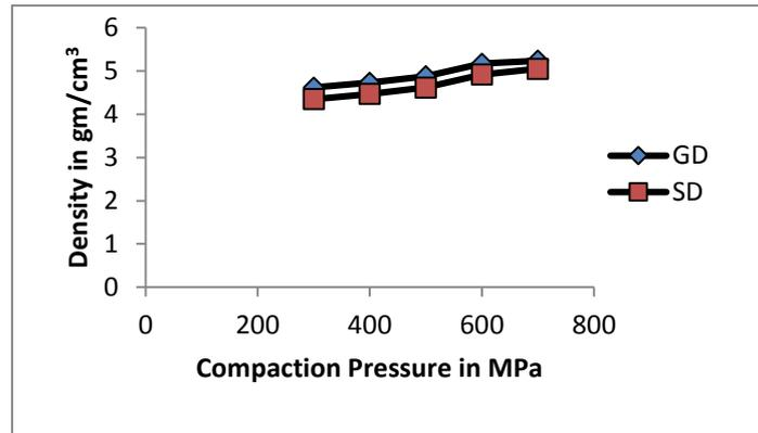
**Figure 1:** Green density and 720<sup>o</sup>C sintered density of the processed material at various compaction pressures.
