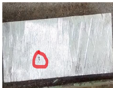
Figure: 5.2.1 Hardness test specimens
