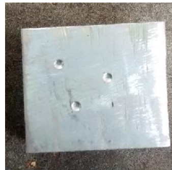
Figure: 5.2.1 Hardness test specimens
