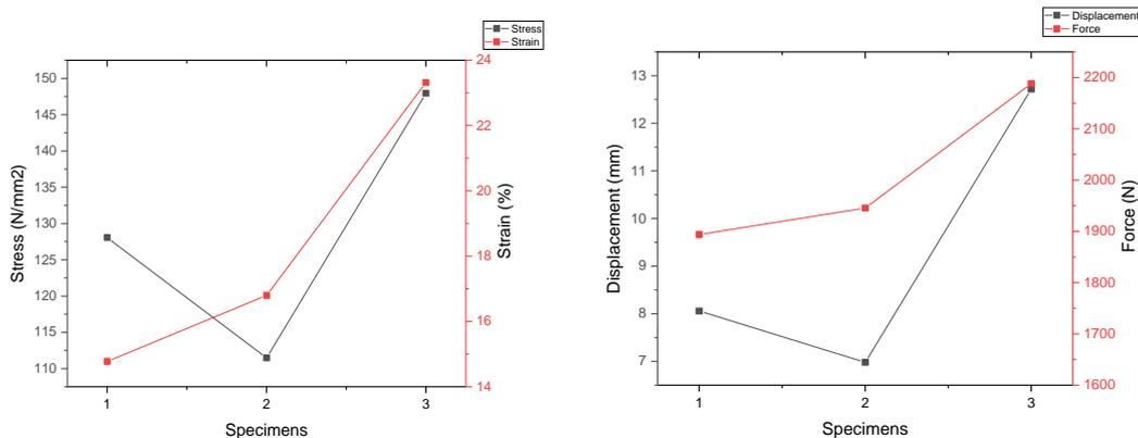
**Figure 4:** Flexural Results - a) Stress-strain curve, b) Load-displacement curve
