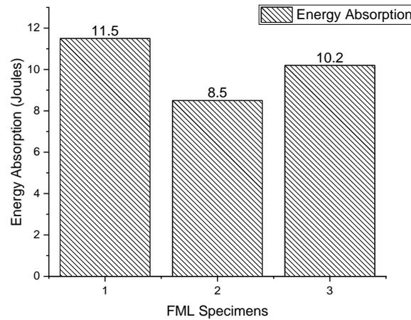
**Figure 5: Izod Impact test results**
