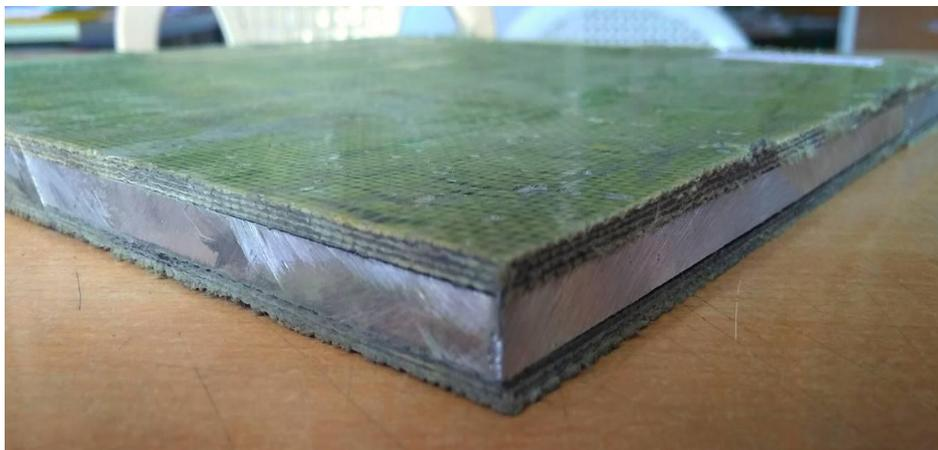
**Figure 1:** Fabricated Sandwich Composite
