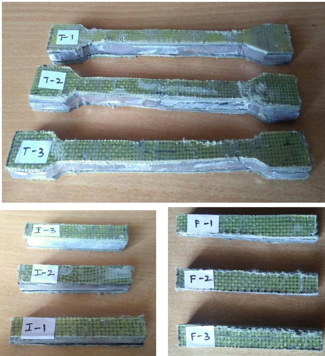
**Figure 2:** Tensile, Izod and Flexural test specimens - Before test
