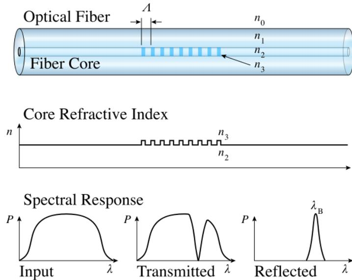
**Fig:** A Fiber Bragg Grating structure, with refractive index profile and spectral response
