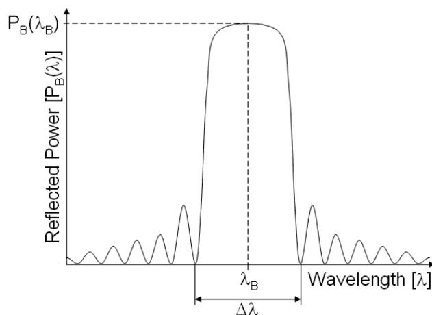
**Fig:** FBG reflected power as a function of wavelength
