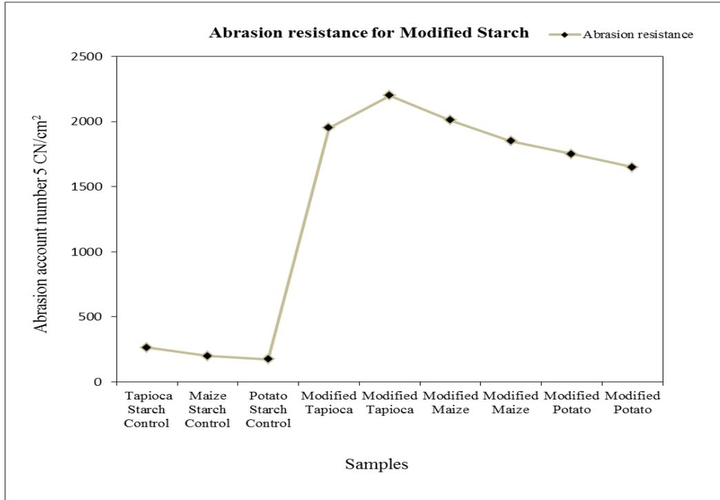
**Graph 2:** Abrasion tested (G552 abrasion tester)
