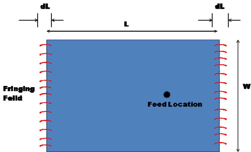
Figure 3: Increase in length of the microstrip patch
