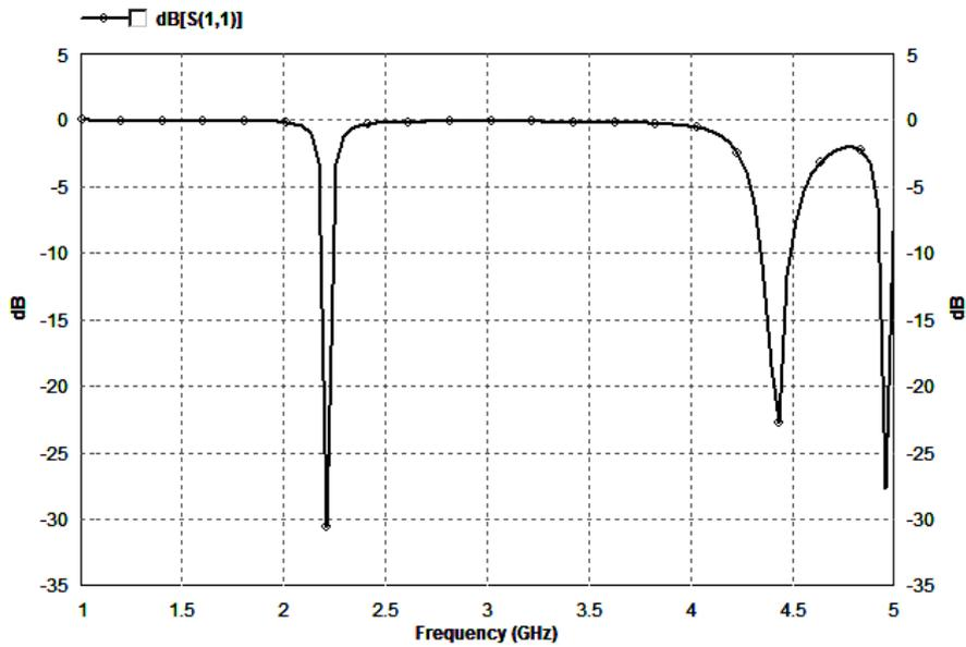
Figure 5: Return loss characteristics at feed point(7,0)
