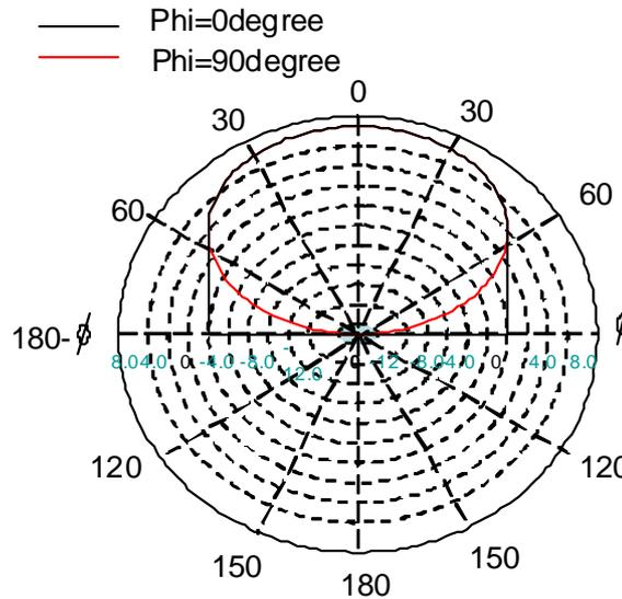
**Figure 6:** Evaluation pattern gain display(dBi)
