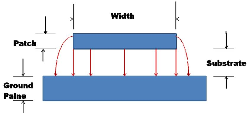
Figure 2: Electric field from a microstrip patch antenna
