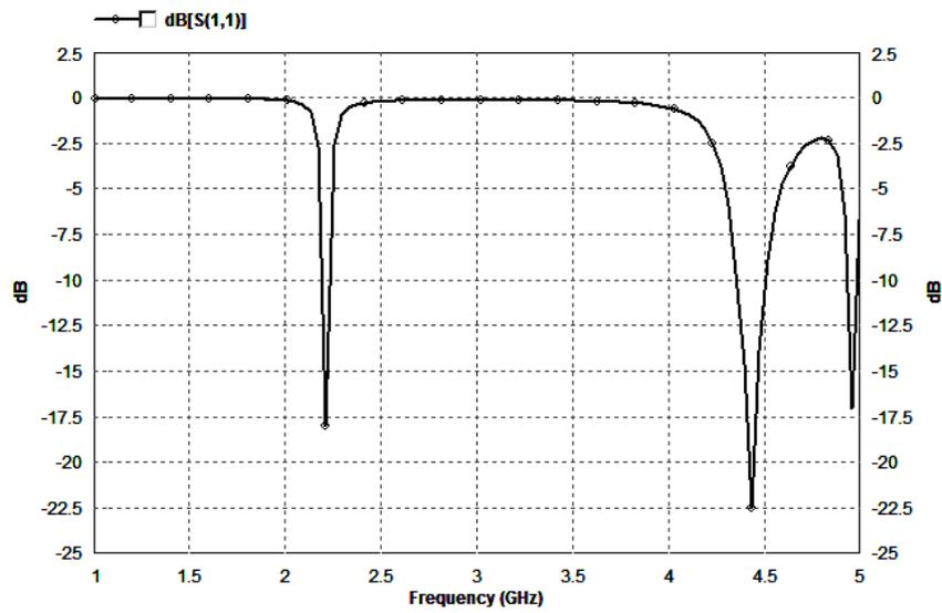
Figure 4: Return loss characteristics at feed point(6,0)
