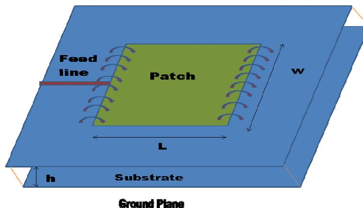
**Figure 1:** Radiation mechanism of microstrip patch
