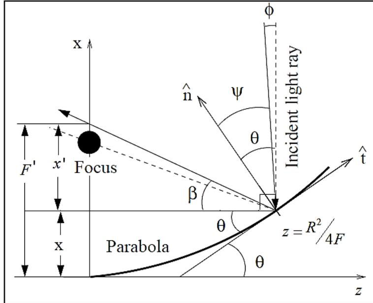
**Fig.2.** Geometry of Parabolic Solar Collector reflected at focal point with misalignment
