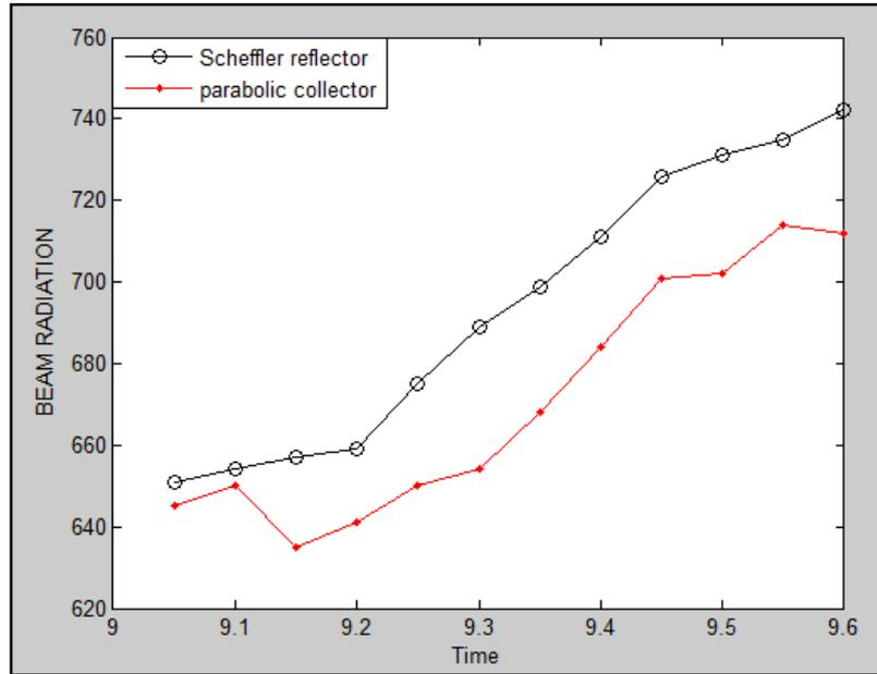
**Fig.7.** Beam Radiation versus time for solar parabolic collector and scheffler reflector
