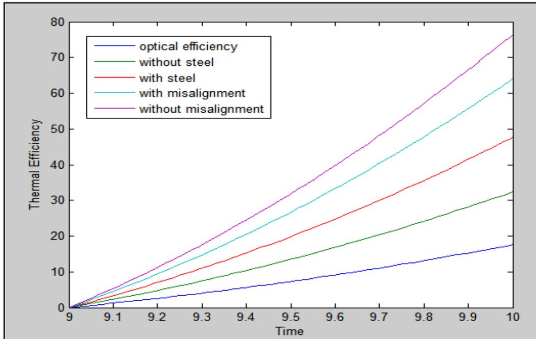
**Fig.11.** Calculated Thermal efficiency of Parabolic Scheffler Reflector with aperture area and radiation as prime parameters
