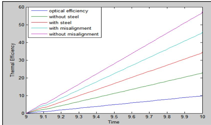
**Fig.9.** Calculated Thermal efficiency of Parabolic Scheffler Reflector with aperture area and radiation as prime parameters
