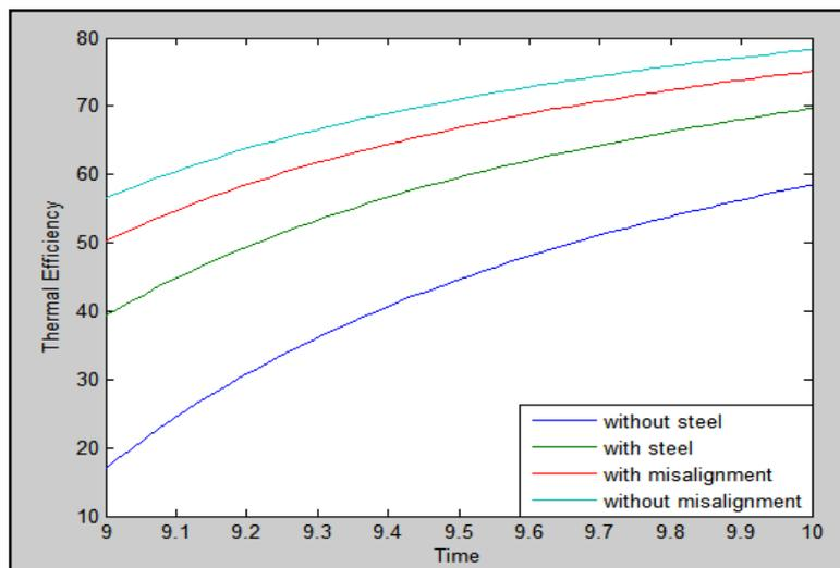
**Fig.10.** Calculated overall efficiency of Parabolic Scheffler Reflector with aperture area and radiation as prime parameters
