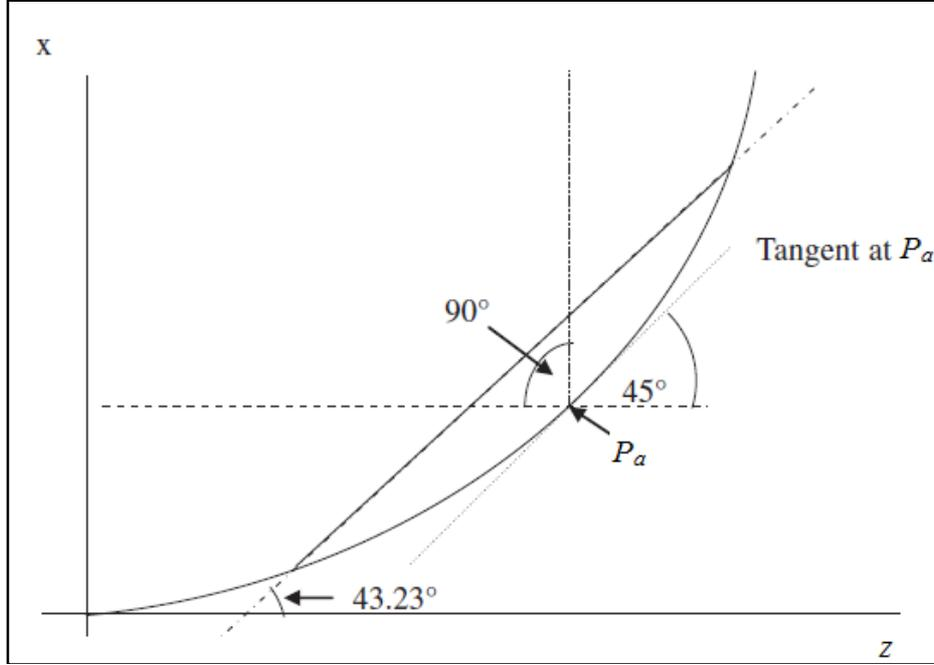
**Fig.3.** Parabolic Reflective Surface of Scheffler
