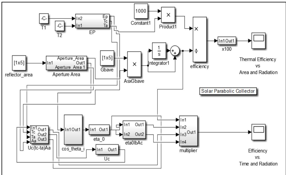
Fig.6. Simulink model for Scheffler Reflector
