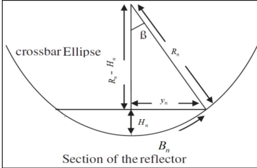
**Fig.4.** Section of Crossbar with the shape of Ellipse
