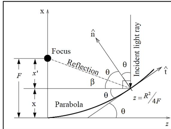
**Fig.1.** Geometry of Parabolic Solar Collector reflected at focal point
