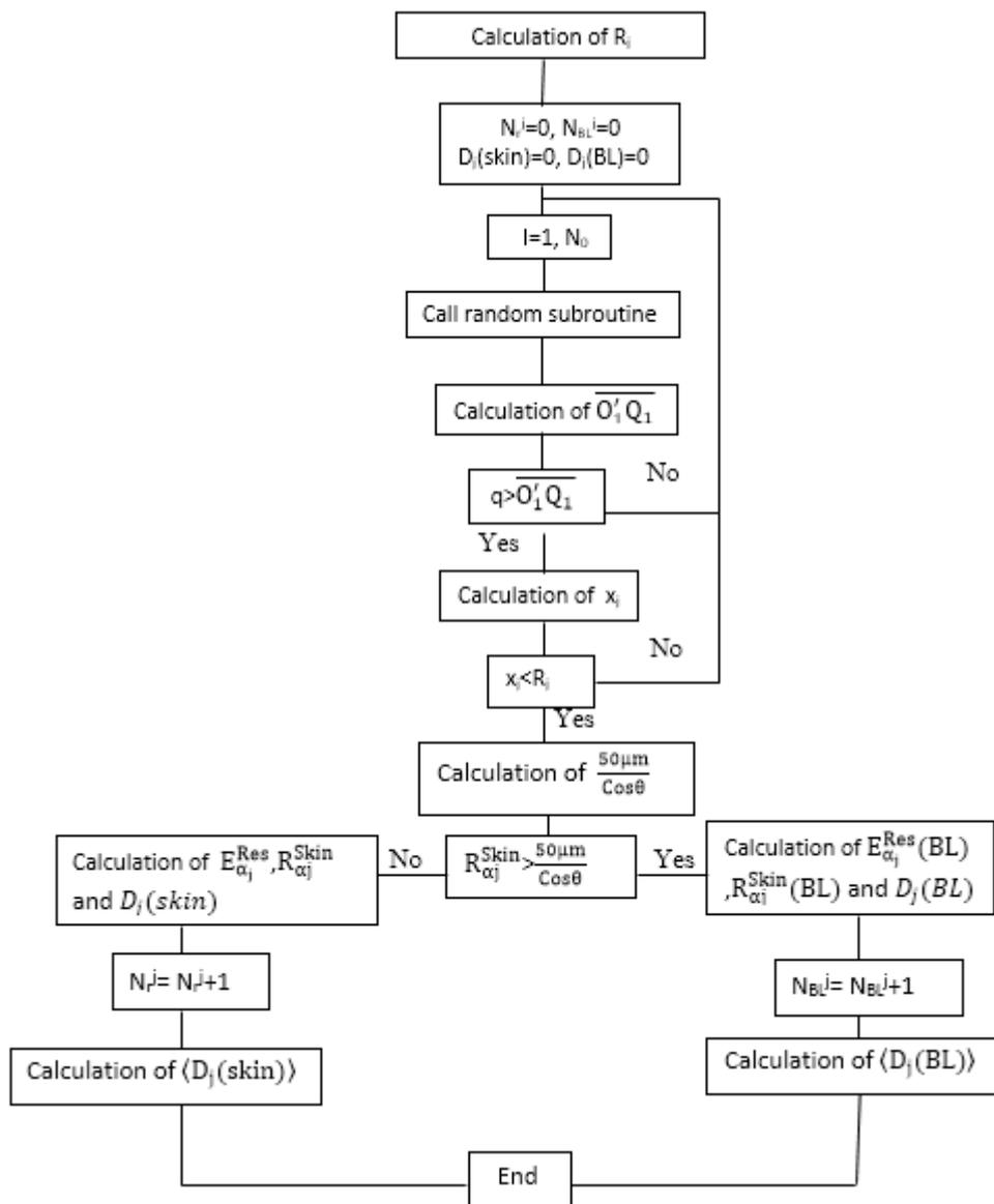
**Fig. 4.** Flow chart of the AMADS Fortran programme which is used to calculate the mean absorbed dose in skin of individuals from deposition of alpha-emitting radionuclides. We employ the same symbols as in the text. It is therefore self-explanatory.  $N_0 = 10^6$  alpha-particles.
