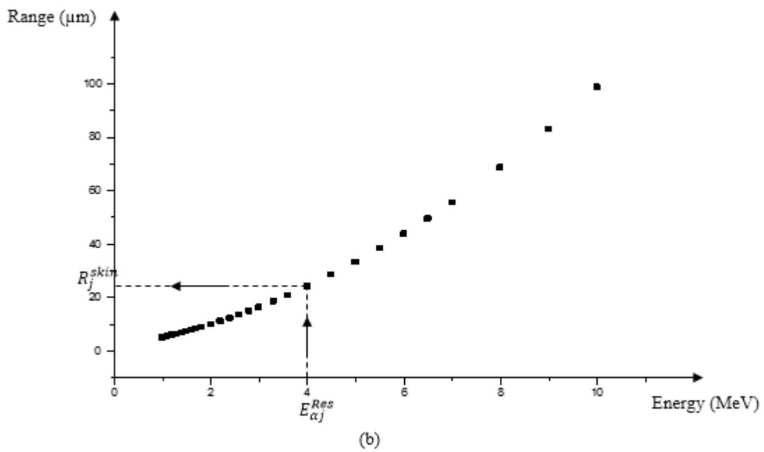
**Fig. 2.** Alpha-particle range-energy relationship for a material sample (a) and skin (b).
