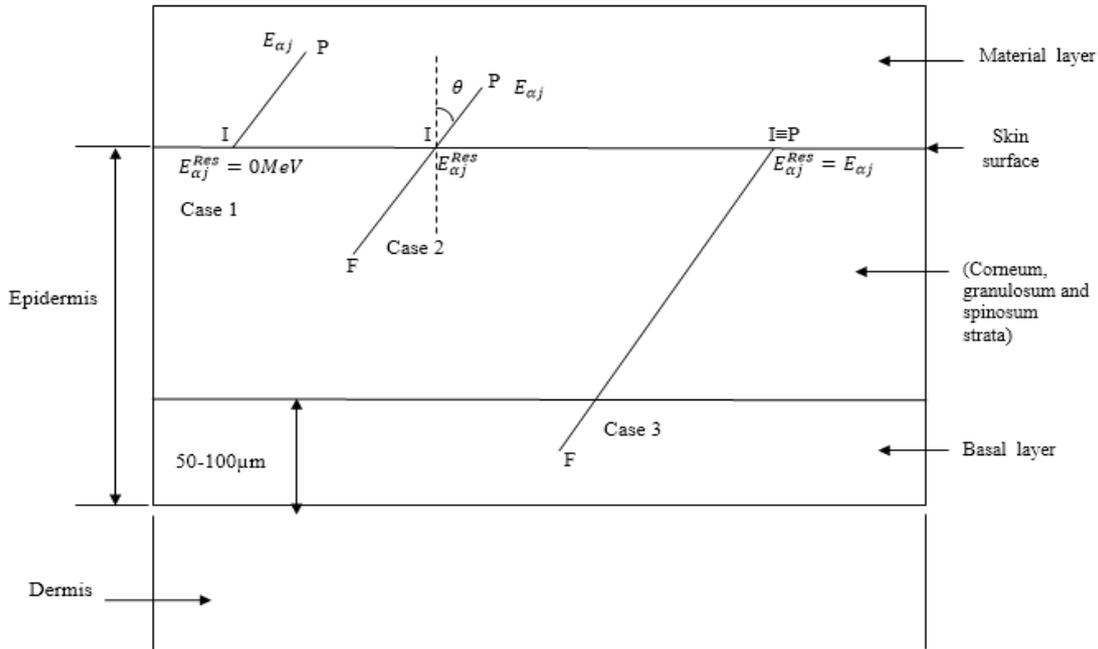
**Fig. 1.** Ranges of an alpha-particle inside a material layer ( $\overline{PI} = x_j$ ) and epidermis ( $\overline{IF} = R_j^{skin}$ ).  $E_{\alpha_j}$  is the initial alpha-particle energy and  $E_{\alpha_j}^{Res}$  its residual energy on the point I. The deposited material layer has a depth of about 1mm.
