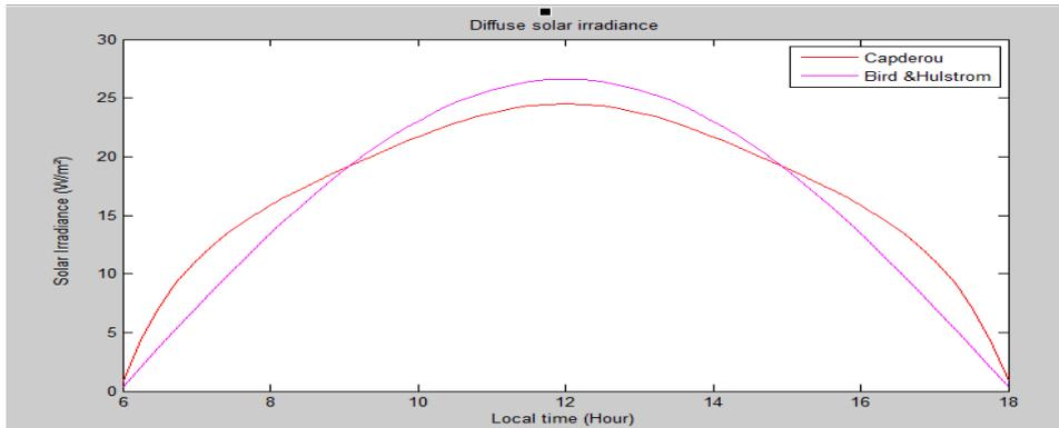
Figure 7: Diffused irradiance estimated under Matlab / Simulink, day of 23/04/1999
