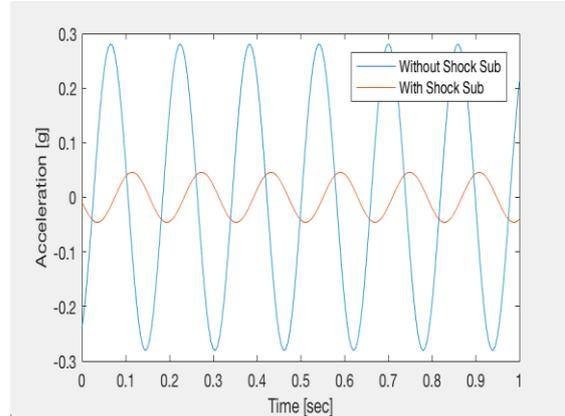
**Figure 5b:** Axial acceleration for 20000lb/in. spring constant at shock sub
