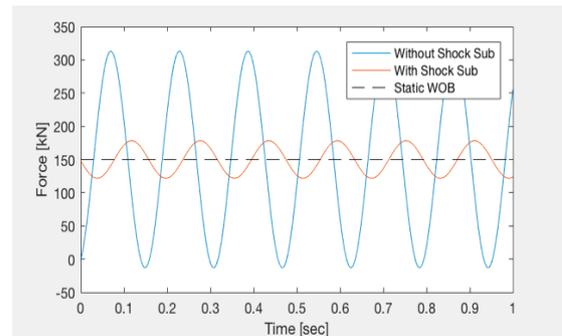
**Figure 4a:** Bit force for 40000lb/in spring constant at shock sub.
