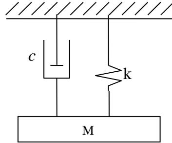
**Figure 2b:** Illustration of Spring-Mass-Dashpot
