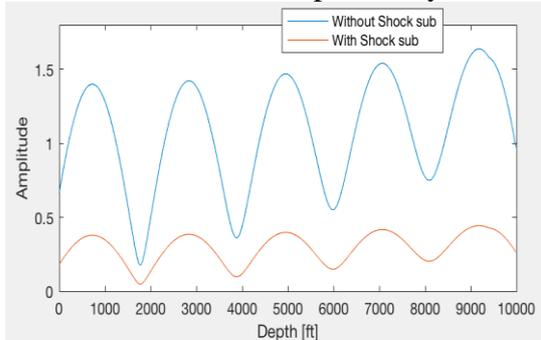
**Figure 3a:** Amplitude with and without shock sub
