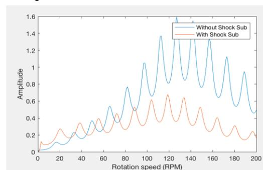
**Figure 3b:** Amplitude as a function of RPM with and without shock sub
