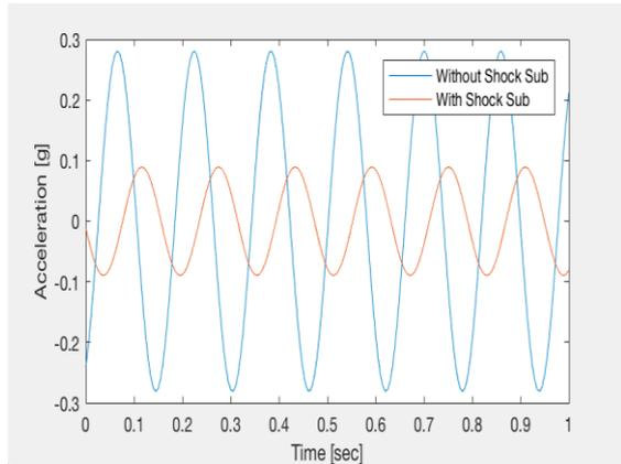
**Figure 5a:** Axial acceleration for 40000lb/in. spring constant at shock sub.
