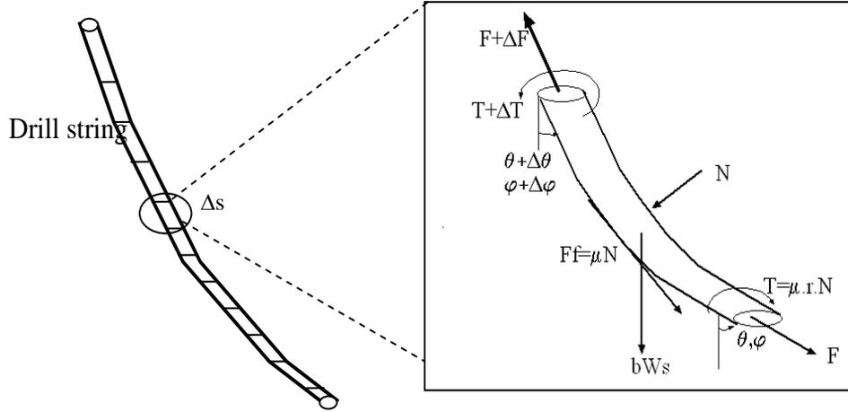
**Figure 1:** Segmented drill string and loads
