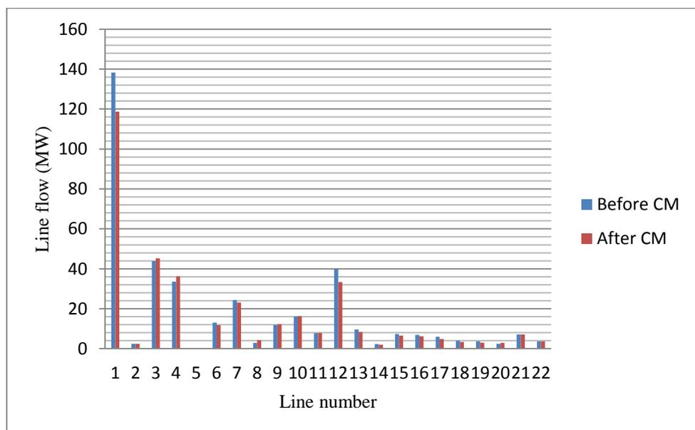
**Figure 3:** Line flow analysis before and after congestion management
