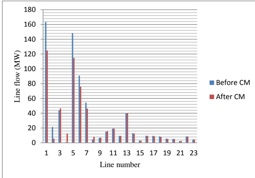
**Figure 1:** Line flow before and after congestion management
