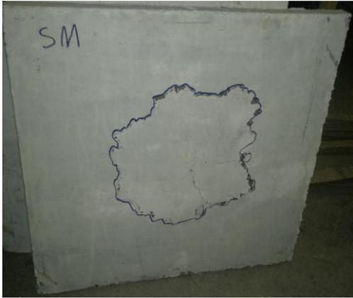
Fig.5 Failure pattern of solid MRPC slab
