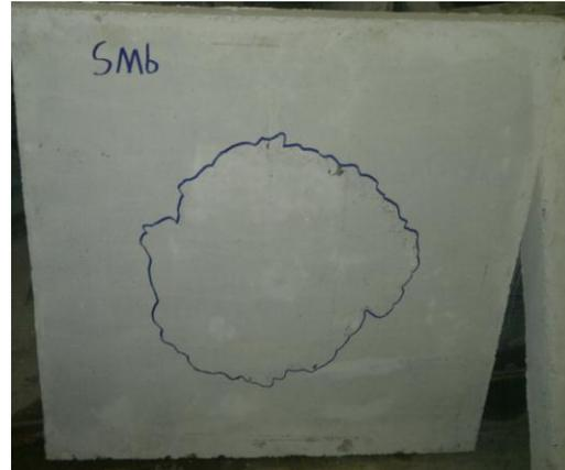
Fig.6 Failure pattern of voided MRPC slab
