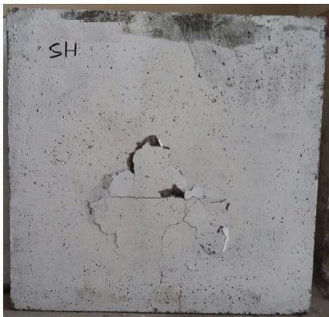
**Fig.3** Failure pattern of solid HSC slab
