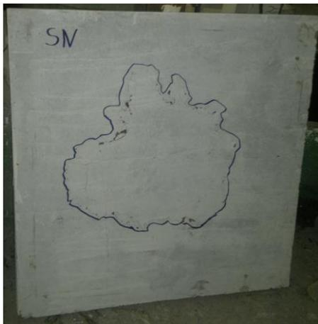
**Fig.1** Failure pattern of solid normal concrete slab
