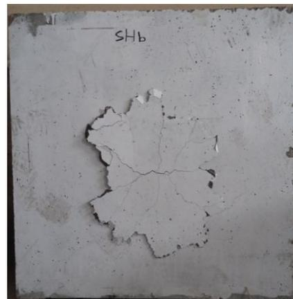
**Fig.4** Failure pattern of voided HSC slab
