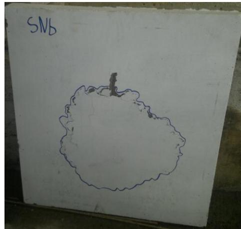
**Fig.2** Failure pattern of voided normal concrete slab
