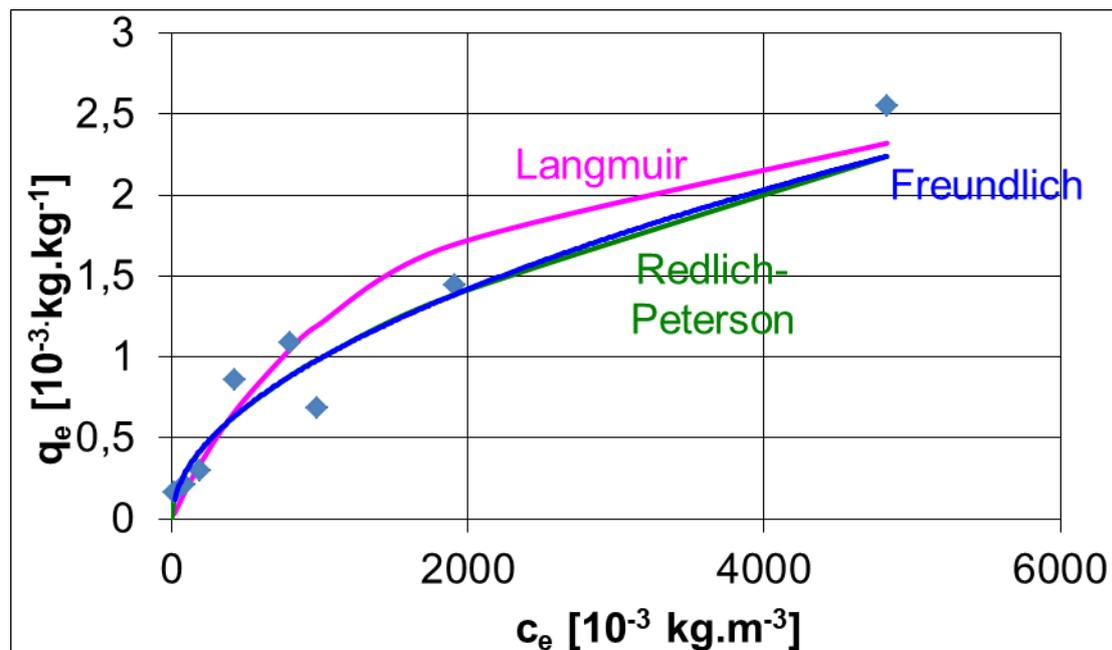
Fig. 3 Adsorption isotherms of Mn on ZeoCem Mn light
