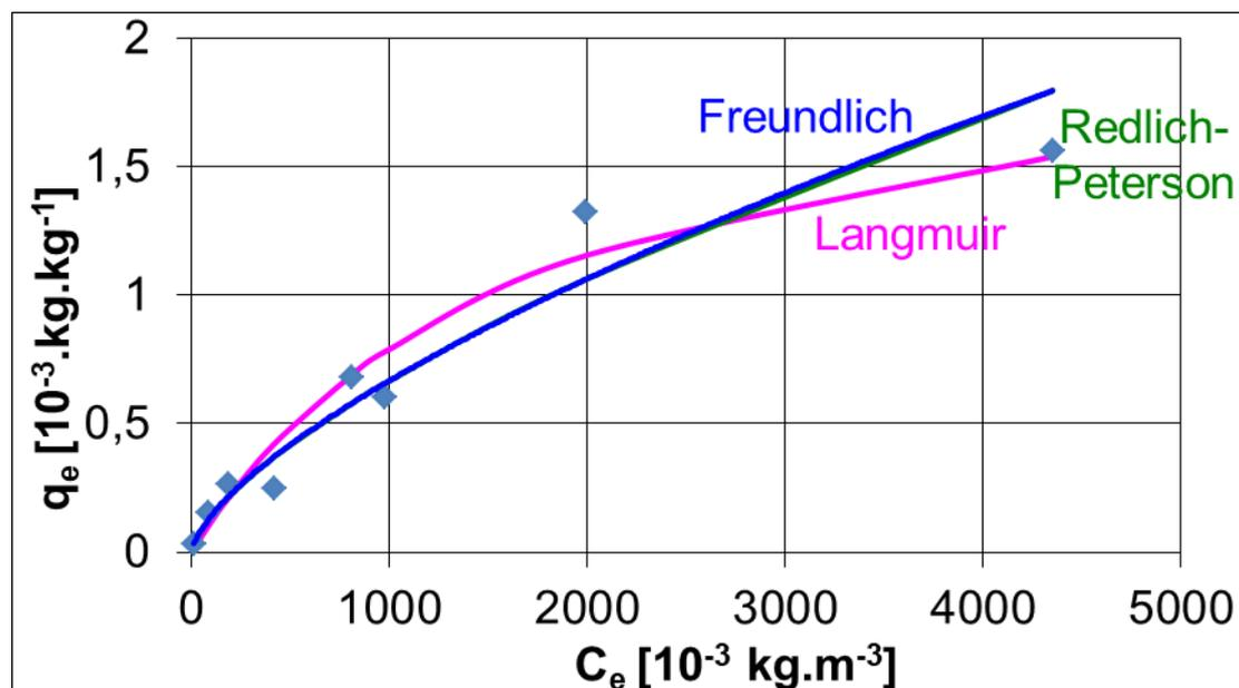
Fig. 2 Adsorption isotherms of Mn on ZeoCem Mn dark
