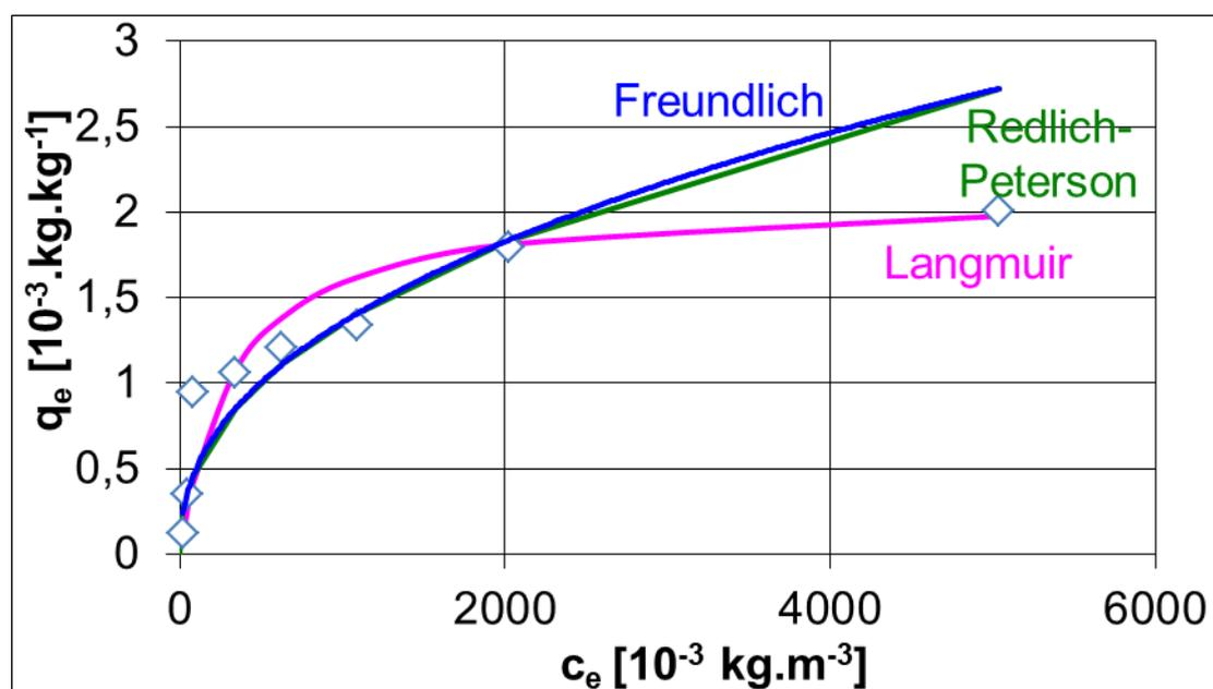
Fig. 4 Adsorption isotherms of Mn on ZeoCem Mn mixed
