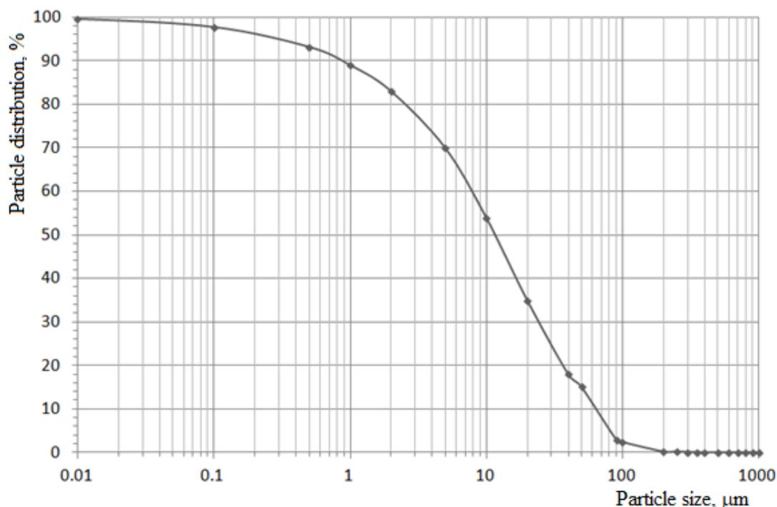
Fig. 1 Particle size distribution of ZeoCem Mn particles [17]
