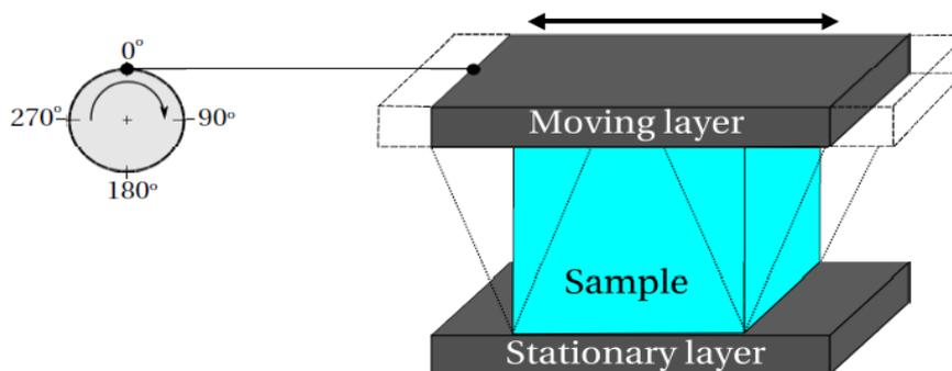
**Figure 1:** Illustration of the two-plate-model oscillatory test [10].
