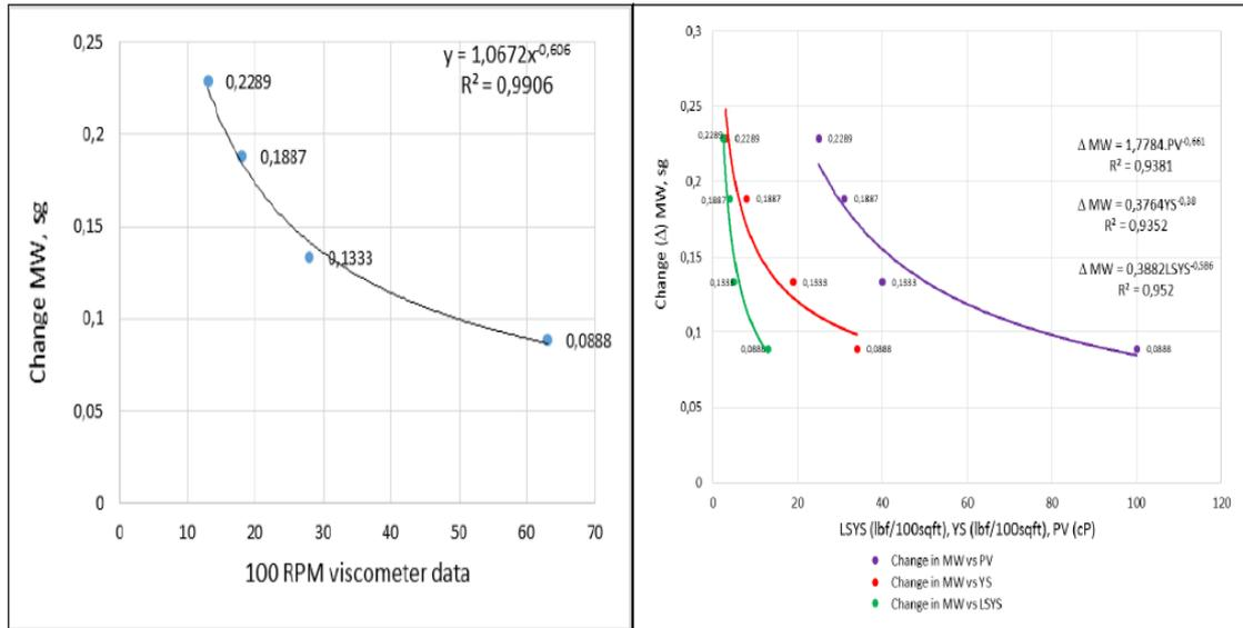
**Figure 8:** Comparisons of change in density and 100RPM viscometer data **Figure 9:** Comparisons of change in density vs PV, YS and LSYS parameter at 50°C
