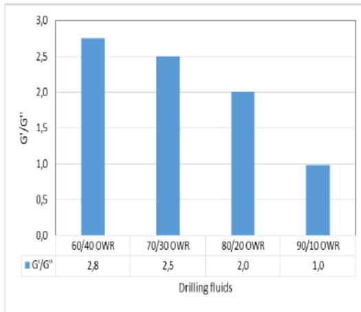
Figure 6:  $G'/G''$  ratio vs OWR at room temperature
