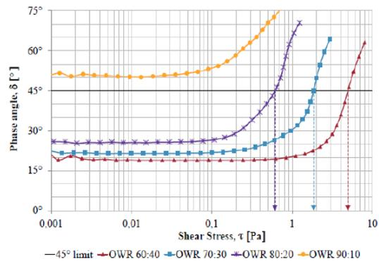
Figure 4: Amplitude sweep test performed on all fluid samples at  $20^{\circ}\text{C}$  and  $\omega = 10\text{rad/s}$ . Note that  $\omega = 20\text{rad/s}$  for the 90:10 sample.
