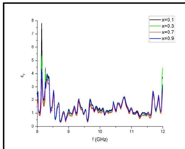
Fig.6 Dielectric Constant as a function of frequency when adding 3g of  $\text{CrMn}_x\text{Ni}_{1-x}\text{FeO}_4$  to rubber paste
