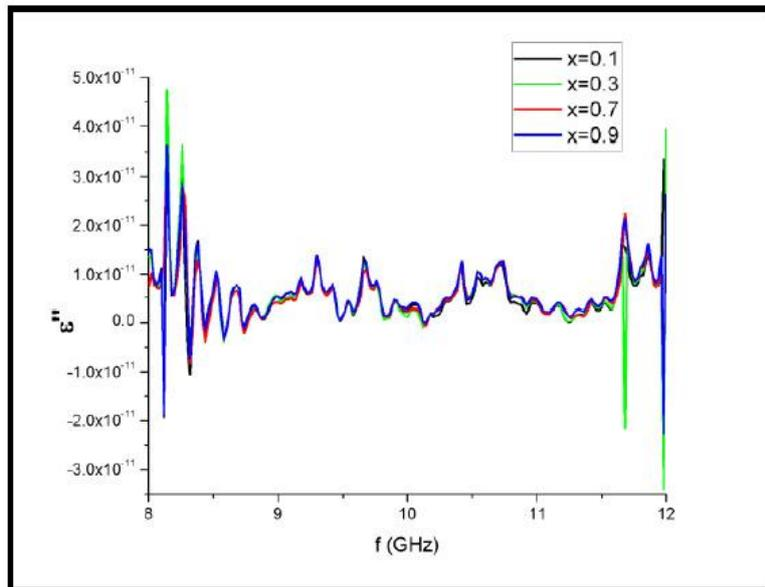
Fig.10 Imaginary part of Permittivity as a function of frequency when adding 3g of  $\text{CrMn}_x\text{Ni}_{1-x}\text{FeO}_4$  to rubber paste
