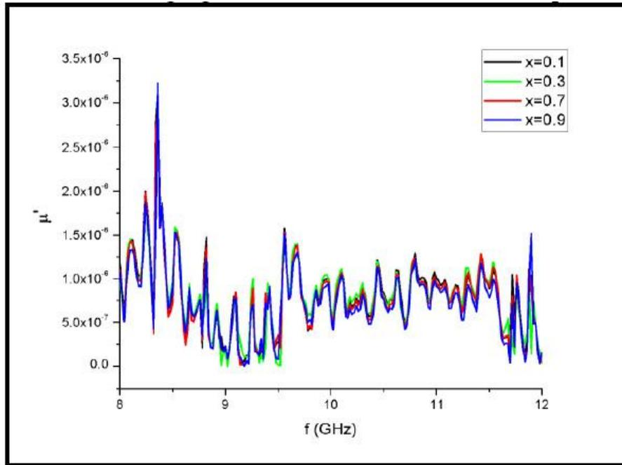
Fig.12 Real part of Relative Permeability as a function of frequency when adding 2g of  $\text{CrMn}_x\text{Ni}_{1-x}\text{FeO}_4$  to rubber paste
