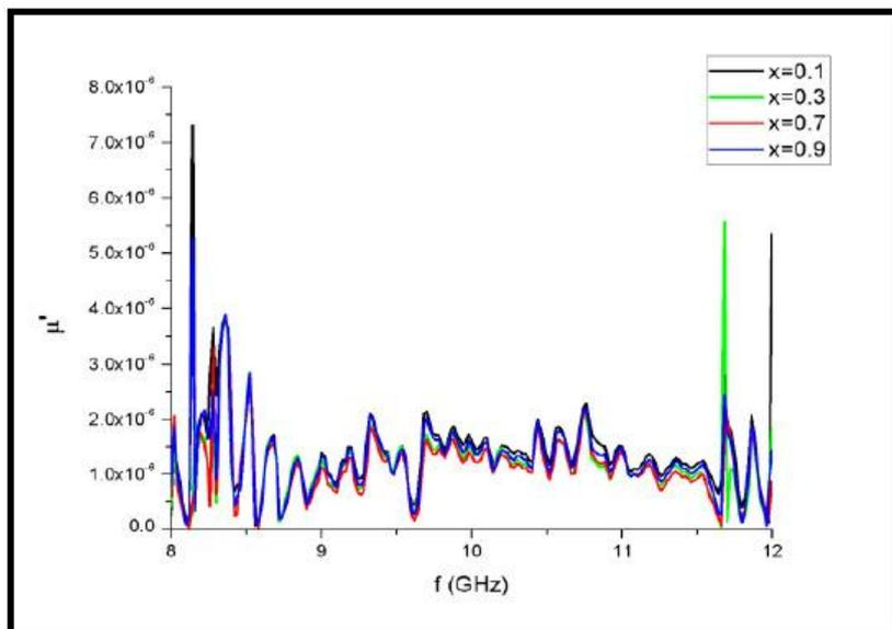
Fig.15 Real part of Relative Permeability as a function of frequency when adding 3g of  $CrMn_xNi_{1-x}FeO_4$  to rubber paste
