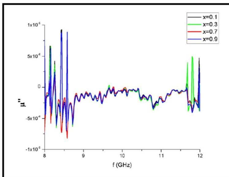
Fig.16 Imaginary part of Relative Permeability as a function of frequency when adding 3g of  $\text{CrMn}_x\text{Ni}_{1-x}\text{FeO}_4$  to rubber paste
