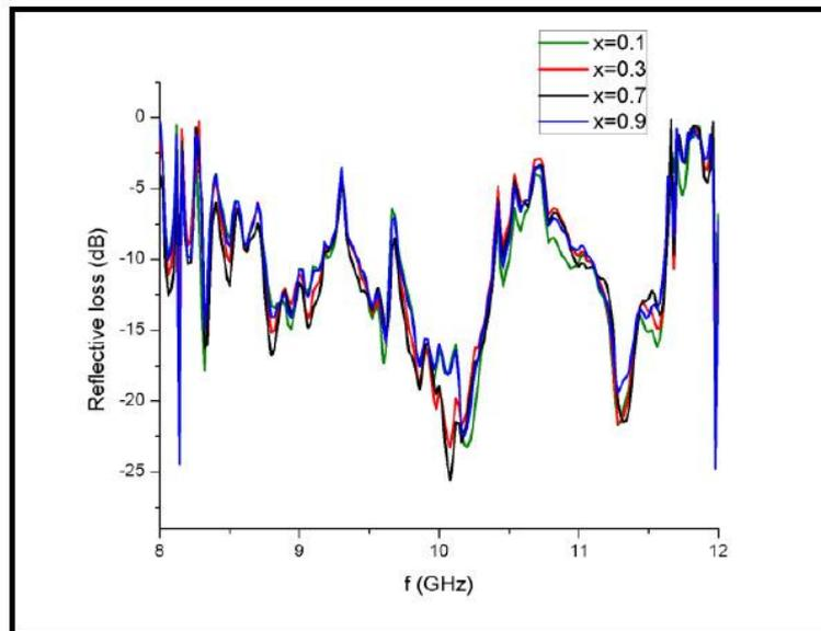
Fig.2 Reflective Loss as a function of frequency, when adding 3g of  $\text{CrMn}_x\text{Ni}_{1-x}\text{FeO}_4$  to rubber paste
