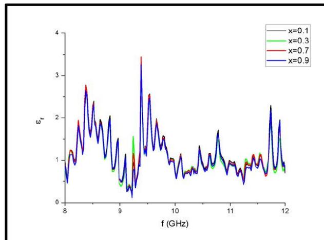
Fig.5 Dielectric Constant as a function of frequency when adding 2g of  $\text{CrMn}_x\text{Ni}_{1-x}\text{FeO}_4$  to rubber paste
