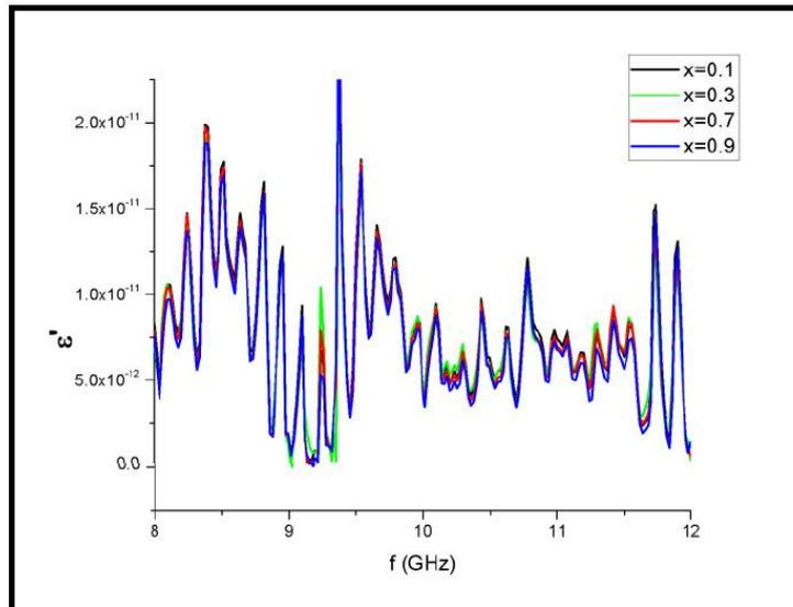
Fig.7 Real part of Permittivity as a function of frequency when adding 2g of  $CrMn_xNi_{1-x}FeO_4$  to rubber paste
