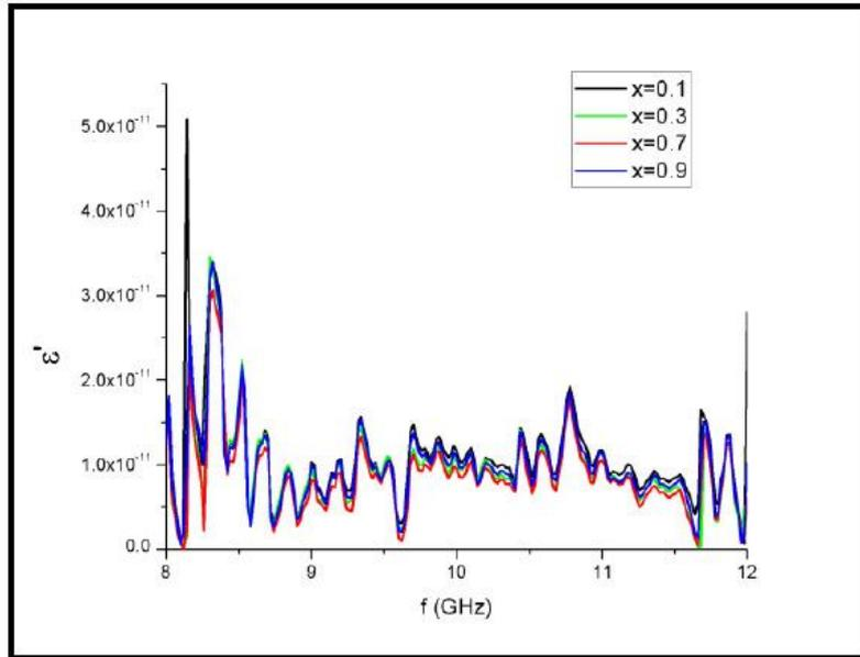
Fig.9 Real part of Permittivity as a function of frequency when adding 3g of  $\text{CrMn}_x\text{Ni}_{1-x}\text{FeO}_4$  to rubber paste
