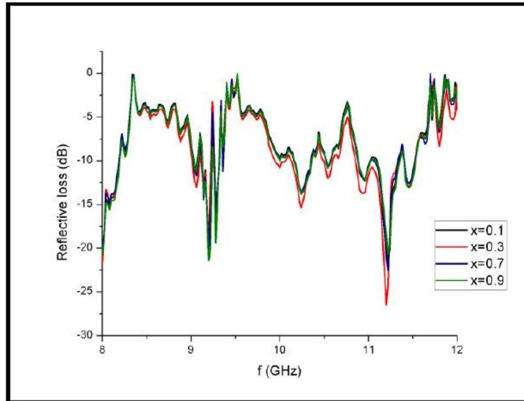
Fig.1 Reflective Loss as a function of frequency, when adding 2g of  $\text{CrMn}_x\text{Ni}_{1-x}\text{FeO}_4$  to rubber paste
