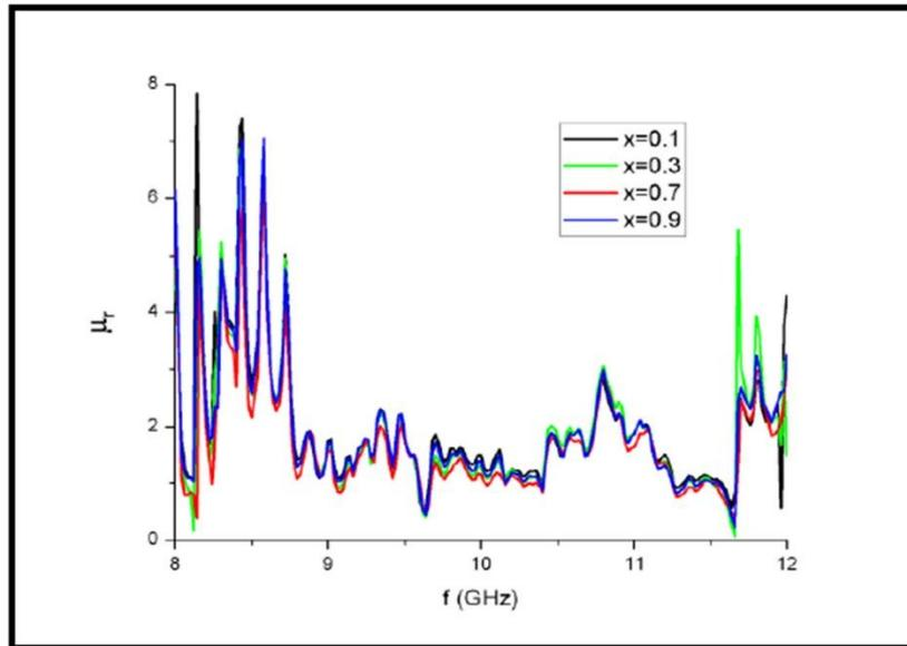
Fig.14 Relative Permeability as a function of frequency when adding 3g of  $CrMn_xNi_{1-x}FeO_4$  to rubber paste
