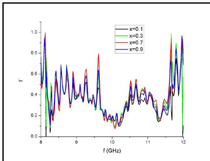
Fig.4 Reflection coefficient as a function of frequency when adding 3g of  $CrMn_xNi_{1-x}FeO_4$  to rubber paste
