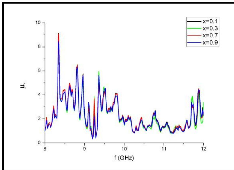
Fig.11 Relative Permeability as a function of frequency when adding 2g of  $CrMn_xNi_{1-x}FeO_4$  to rubber paste
