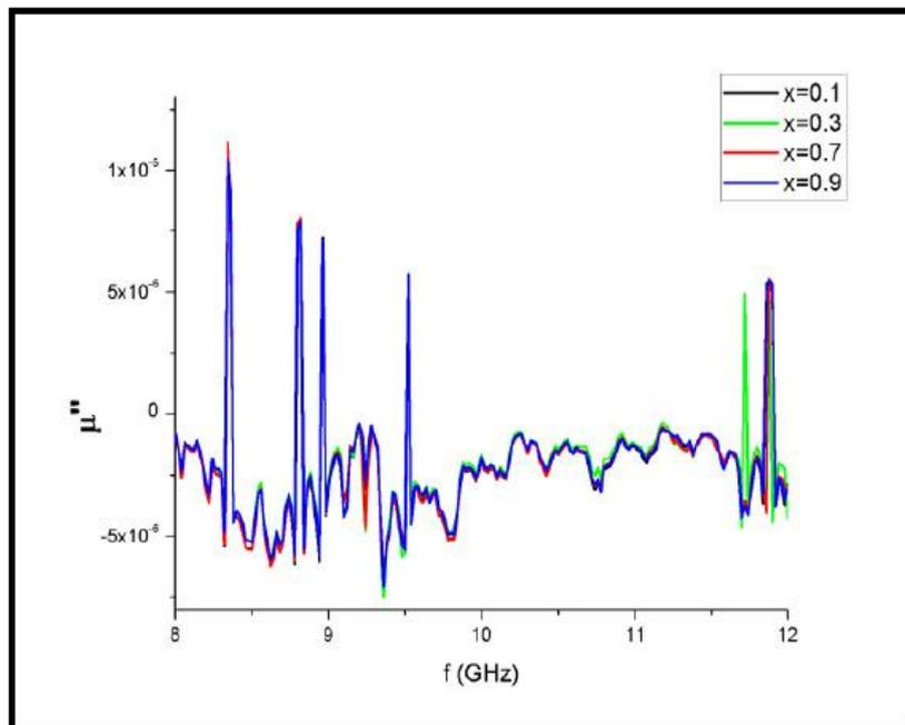
Fig.13 Imaginary part of Relative Permeability as a function of frequency when adding 2g of  $\text{CrMn}_x\text{Ni}_{1-x}\text{FeO}_4$  to rubber paste
