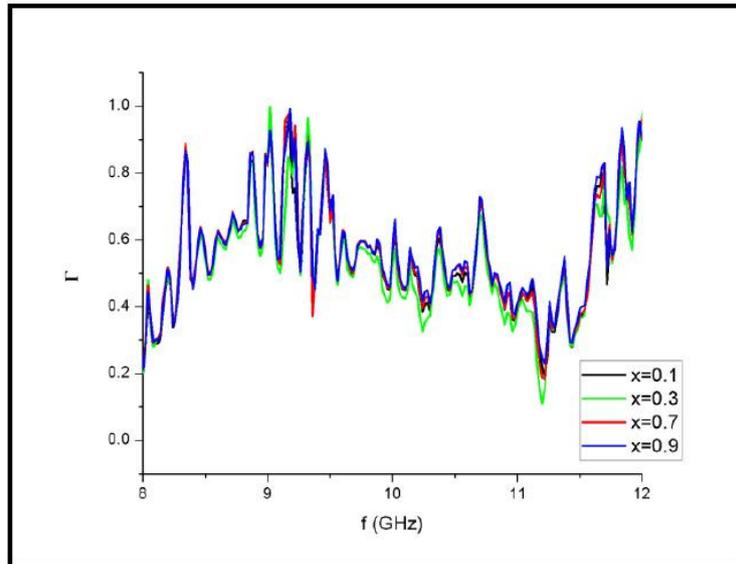
Fig.3 Reflection coefficient as a function of frequency when adding 2g of  $CrMn_xNi_{1-x}FeO_4$  to rubber paste
