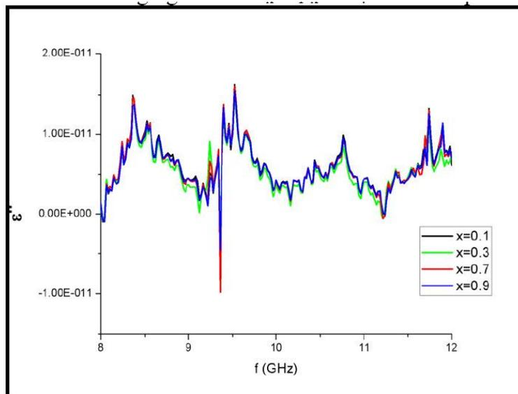
Fig.8 Imaginary part of Permittivity as a function of frequency when adding 2g of  $CrMn_xNi_{1-x}FeO_4$  to rubber paste
