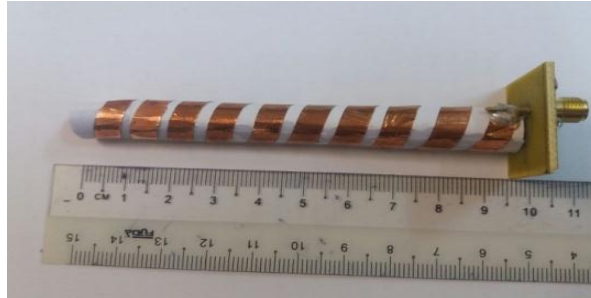
Figure 8: Fabricated design of 10 GHz helical antenna using Paper material
