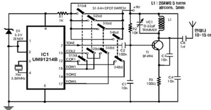
Fig. 4 Wireless transmit circuit schematic diagram
