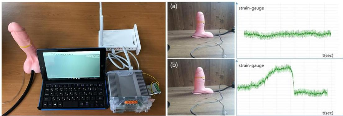
**Fig. 8** Date graph of strain gauge achieved: (a) before erection (b) after erection
