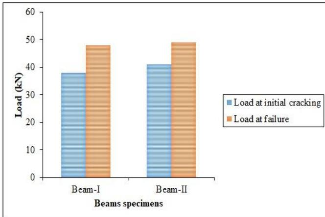
Fig. 3. Load carrying capacity for Beam-I and Beam-II
