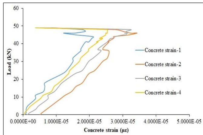
Fig. 7. Load versus concrete strain for Beam-II
