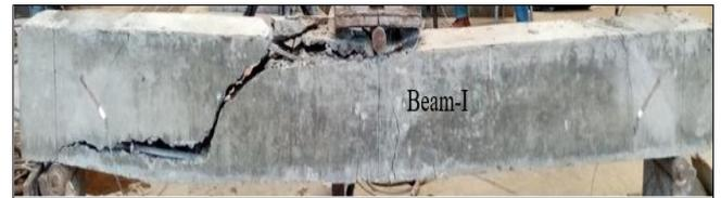
Fig. 8. Crack and failure pattern of Beam-I after testing
