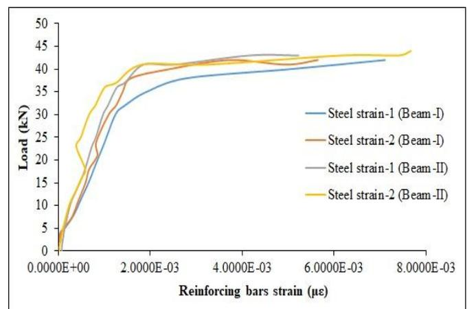
Fig. 5. Load versus reinforcing bars strain for Beam-I and Beam-II specimens
