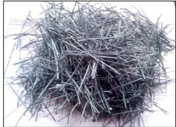
Fig. 1. Recycled tyres steel fibres
