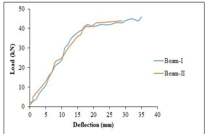
Fig. 4. Load versus deflection curves for Beam-I and Beam-II specimens
