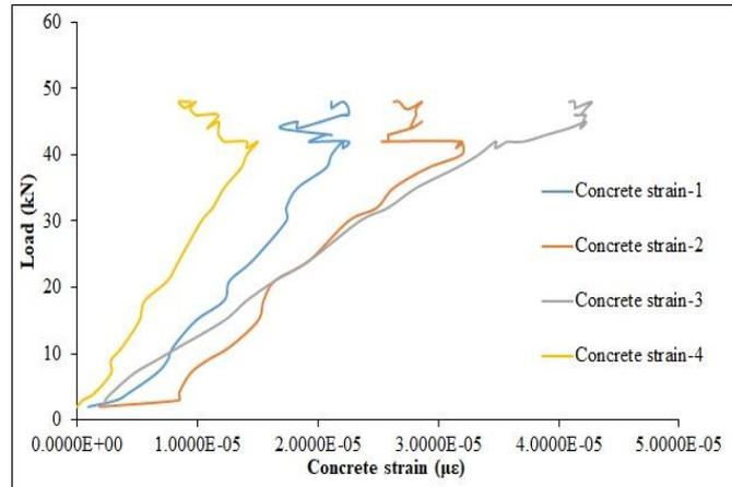
Fig. 6. Load versus concrete strain for Beam-I
