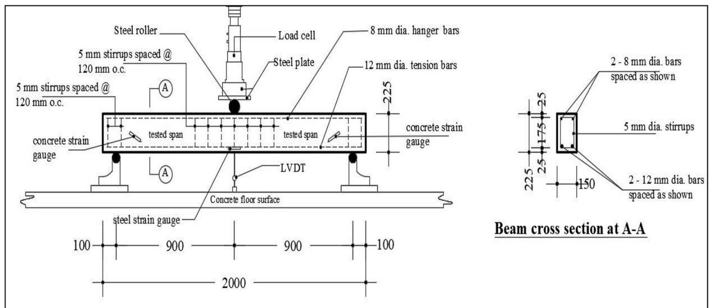
**Fig. 2.** Experimental setup and reinforcing bars details for Beam-I and Beam-II specimens
