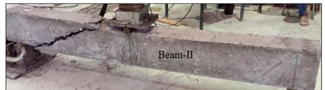
Fig. 9. Crack and failure pattern of Beam-II after testing
