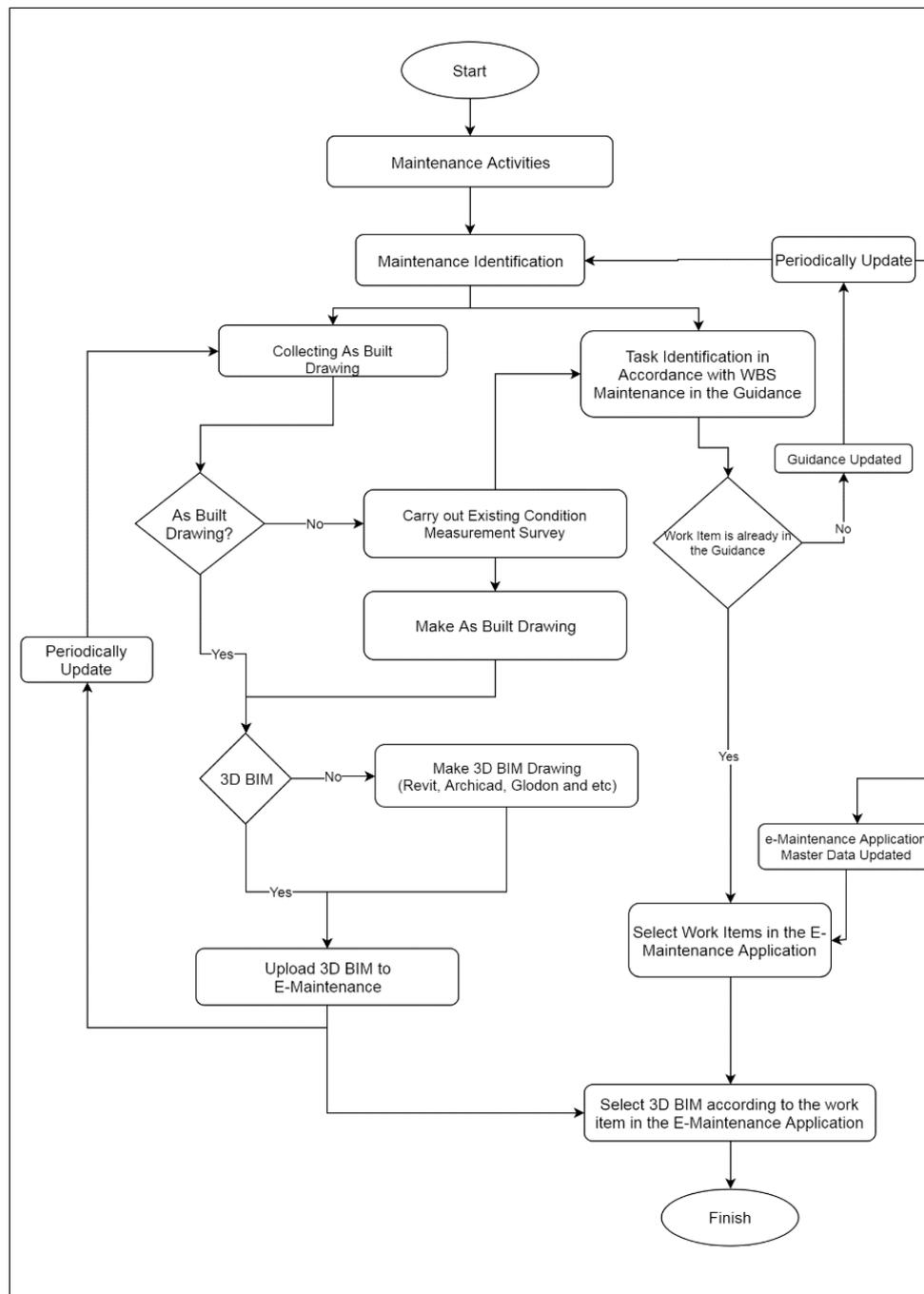
**Fig. 5** Information System Development (E-Maintenance) Flowchart Based on WBS by using BIM
