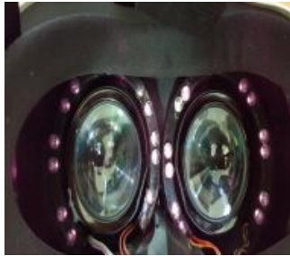
Fig. 2. Addition of the hardware infrared camera
