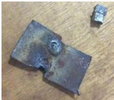
**Figure 4:** Mild Steel Weld joint
