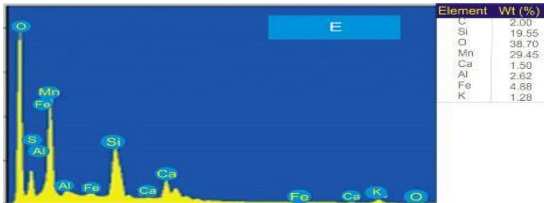
**Figure 11:** EDS graph of Nano flux welding powder
