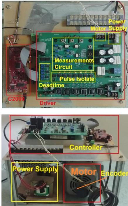
Figure 4. Controller and driver
