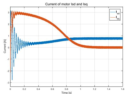
Figure 7. Experimental results of  $I_{dq}$  of the magnetic flux model
