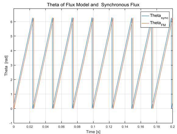
Figure 6. Experimental results of measuring the magnetic flux angle
