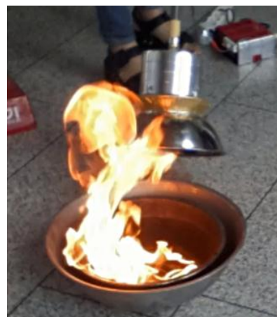
Fig 1. Sound Fire Extinguisher from SSERI [4]
