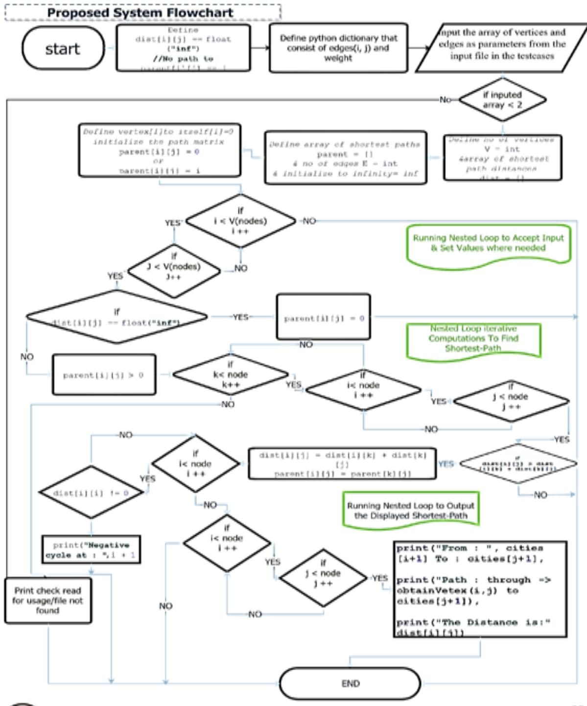
Figure 1: Flowchart Application of proposed Floyd-Warshalls Algorithm for Air-Freight Service
