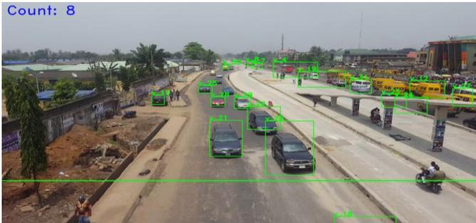
**Figure 7:** Tracking multiple vehicles with the DCF-CSR
