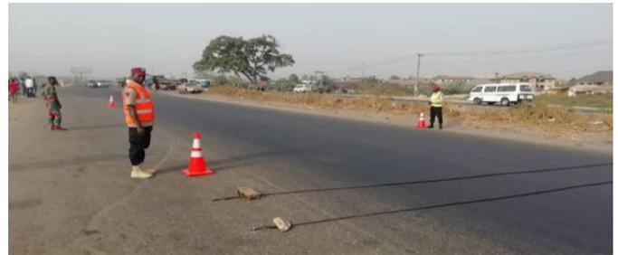
**Figure 1:** FRSC personnel using the MetroCount pneumatic road tube counter to record traffic count along the Lagos-Ibadan expressway (Federal Road Safety Corps, 2019)
