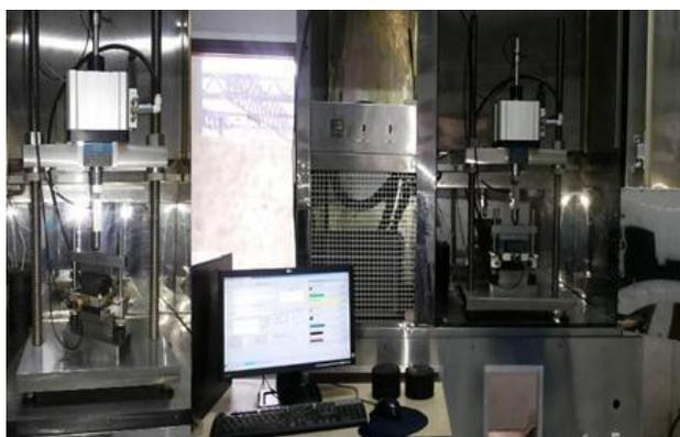
**Fig. 2.** Test device for resilient modulus.
