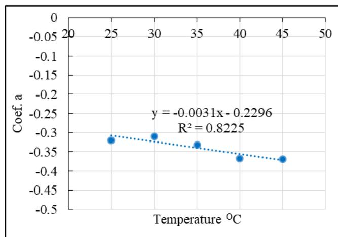
**Fig. 7.** Relationship between temperature and a coefficient regression of asphalt penetration index.
