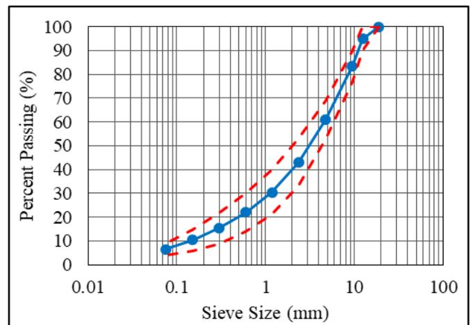
Fig. 1. Aggregate gradation type used in the study.
