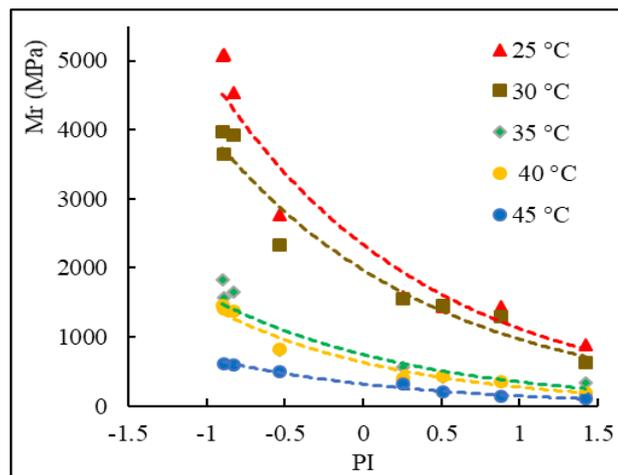
**Fig. 5.** Relationship between resilient modulus and PI.
