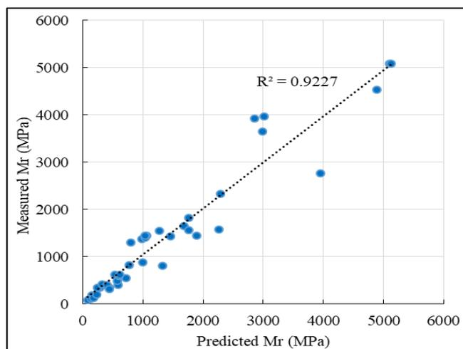
**Fig. 9.** Experimental results versus model predicted  $M_r$ .
