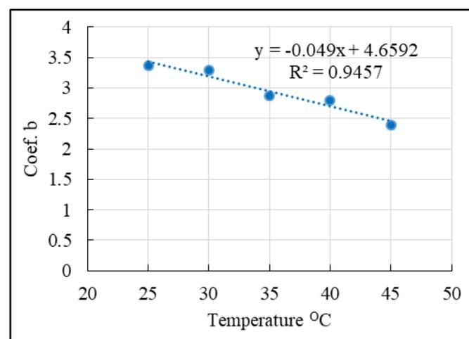
**Fig. 8.** Relationship between temperature and b coefficient regression of asphalt penetration index.
