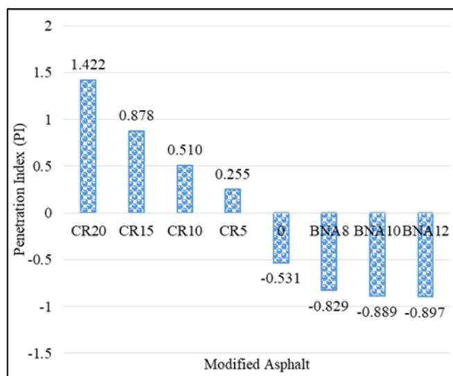
**Fig. 3.** Penetration index value on various modified asphalt.
