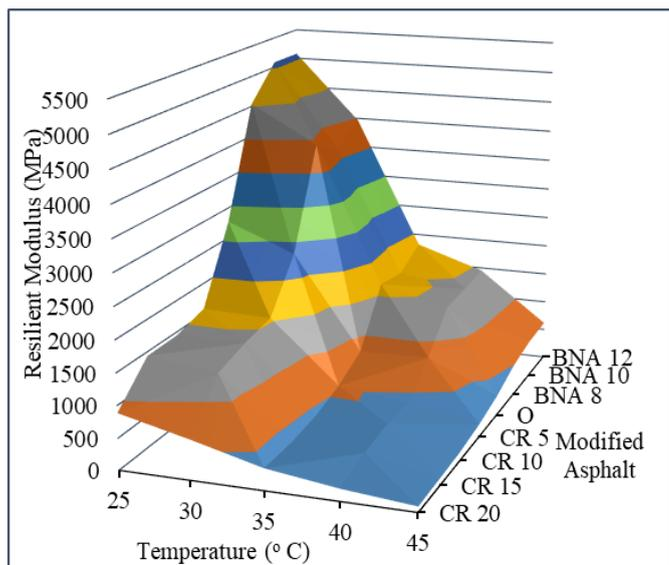
**Fig. 4.** Resilient modulus on various modified asphalt and temperatures.
