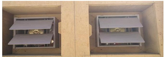
**Fig. 3.** The two suction fans fitted on the test chamber
