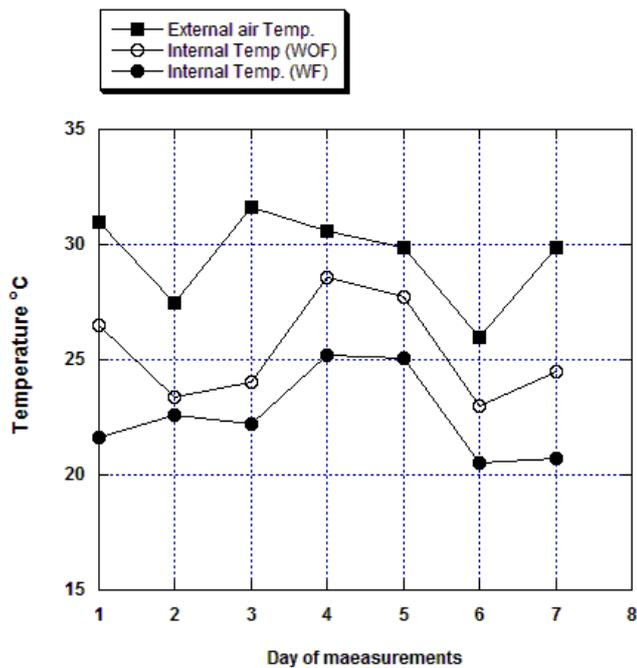
**Fig. 6.** External and internal temperature distribution with/without induced fans
