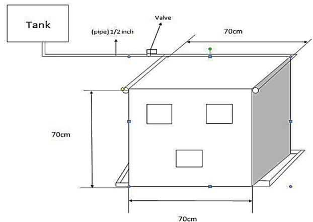
**Fig. 4.** A sketch of the designed model with a drainage system
