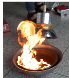
Fig 1. Sound Fire Extinguisher
