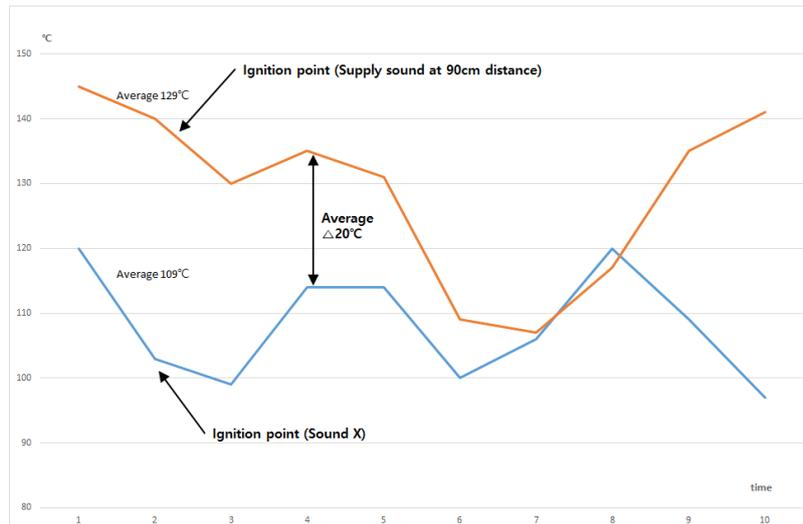
**Fig 4.** Measurement result of ignition point of matches
