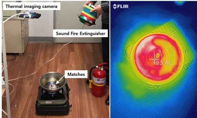
**Fig 2.** Experiment scene and thermal image recording screen
