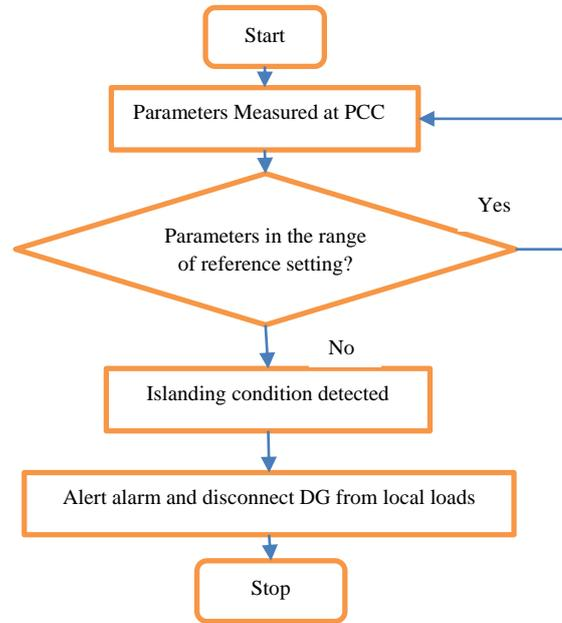
**Figure 4:** Flow chart for passive method
