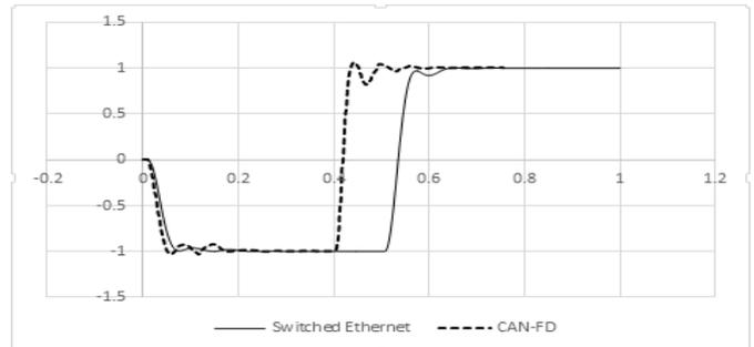
**Fig. 5:** CAN-FD and 100M Switched Ethernet networks with probability loss of 5%
