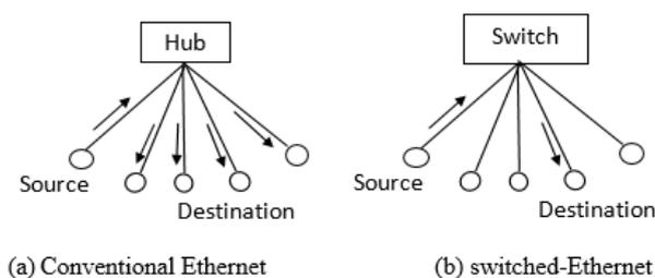
Fig. 1: Comparison of transmission method of Ethernet and 100M Switched Ethernet. Fig. 1 illustrates the operations of hubs and switches when used with Ethernet.
