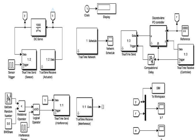
Fig. 3: NCS Model. Fig. 3 shows the NCS in-built model by Truetime kernel in the environment of Matlab/ Simulink 16b.
