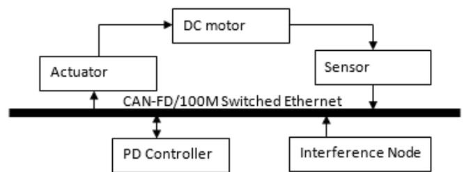
Fig. 2: A block diagram model of the NCSs. Fig. 2 illustrates how the different control components are interconnected through the network.
