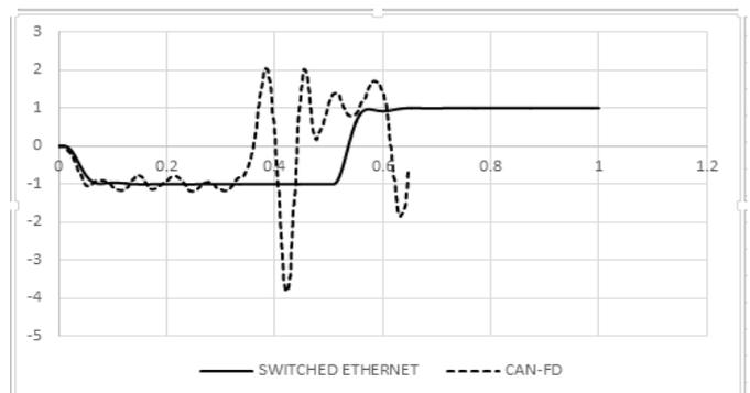
**Fig. 12:** Simulation results for each network when real-time network process is shared with other applications with an interference of 50%.
