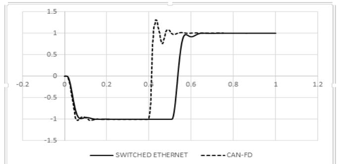
**Fig. 11:** Simulation results for each network when real-time network process is shared with other applications with an interference of 30%.
