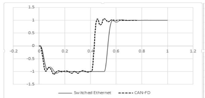
**Fig. 6:** CAN-FD and 100M Switched Ethernet networks with probability loss of 10%
