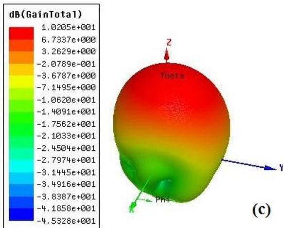
**Fig. 5** Simulation results of the conventional MS 2x2 MPAA of configuration 1 (a). Return loss  $S_{11}$  versus frequency (b). Radiation pattern of the gain in E plane ( $\phi=0^\circ$ ) (c). 3D polar plot of the antenna gain
