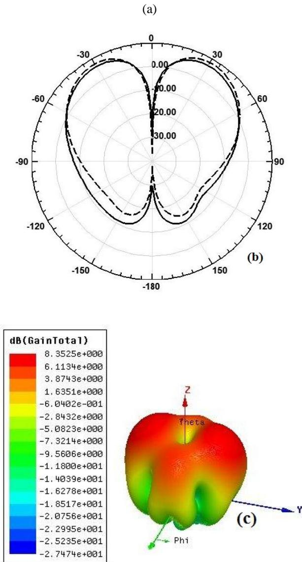
**Fig. 7** Measured results of the fabrication 2x2 MS MPA array (configuration 2) (a). Return loss  $S_{11}$  versus frequency (b). Radiation pattern of the gain in E-plane ( $\phi=0^\circ$ ) (c). 3D polar plot of the antenna gain
