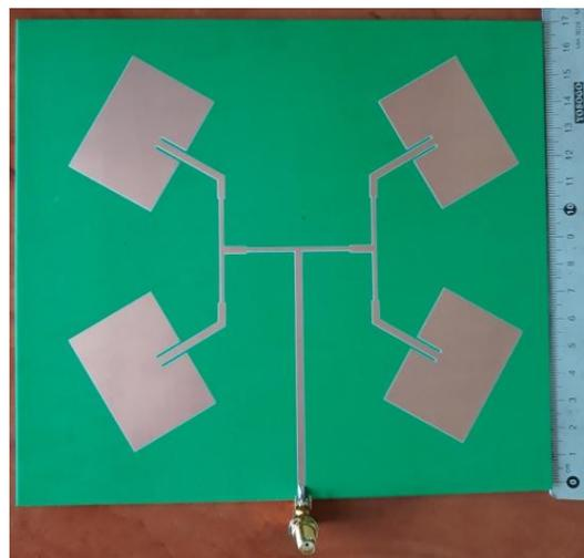
**Fig. 6** Fabricated conventional MS 2x2 MPAA array (configuration 2)
