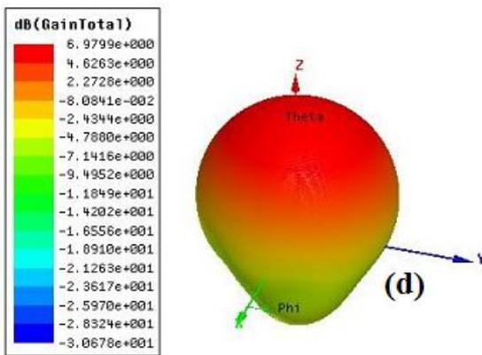
**Fig. 8** Simulation results of SMS 2×2 MPA array (configuration 1) (a). Ansoft HFSS photograph of the SMS array (configuration 1) (b). Return loss  $S_{11}$  versus frequency (c). Radiation pattern of the gain in E plane ( $\phi=0^\circ$ ) (d). 3D polar plot of the antenna gain
