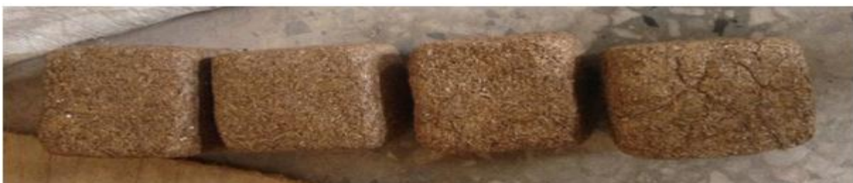
Fig. 3. Briquettes produced using the briquetting machine
