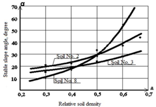
**Fig. 3.** Dependence of stable slope steepness on the relative density of loess soils
