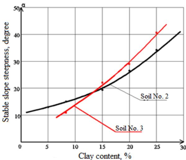
Fig. 5. Dependence of stable slope steepness on clay content in soil
