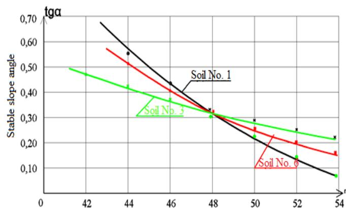
**Fig. 2.** Dependence of stable slope steepness on soil porosity
