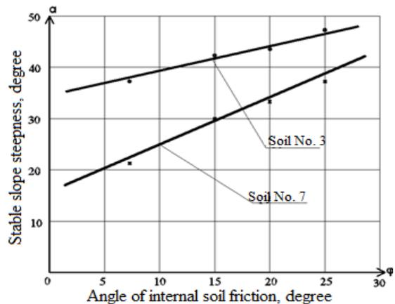
**Fig. 4.** Dependence of stable slope steepness on the angle of internal soil friction
