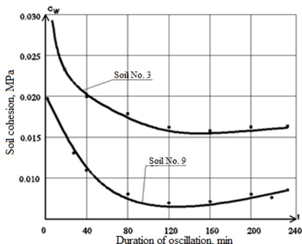
Fig. 8. The nature of changes in soil cohesion in time during the oscillation process with the acceleration  $\lambda_c=2000\text{mm/s}^2$
