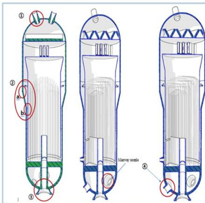
**Figure 1.** Manway nozzle under investigation shown on the model in the center
