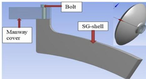
**Figure 2.** A 3-D model for the manway nozzle
