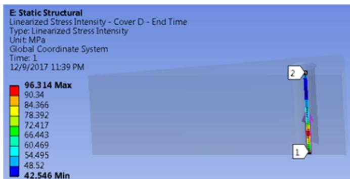
**Figure 9** Sample stress path result for blind under level A analysis
