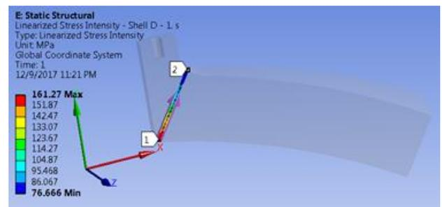
**Figure 8** Sample stress path result for Shell under level A analysis
