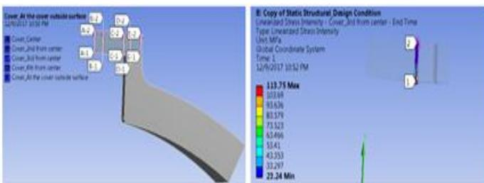
**Figure 6** Location of stress paths and results for stresses along path D on blind cover
