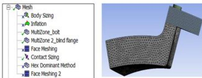
**Figure 3.** Meshing techniques used and meshed model
